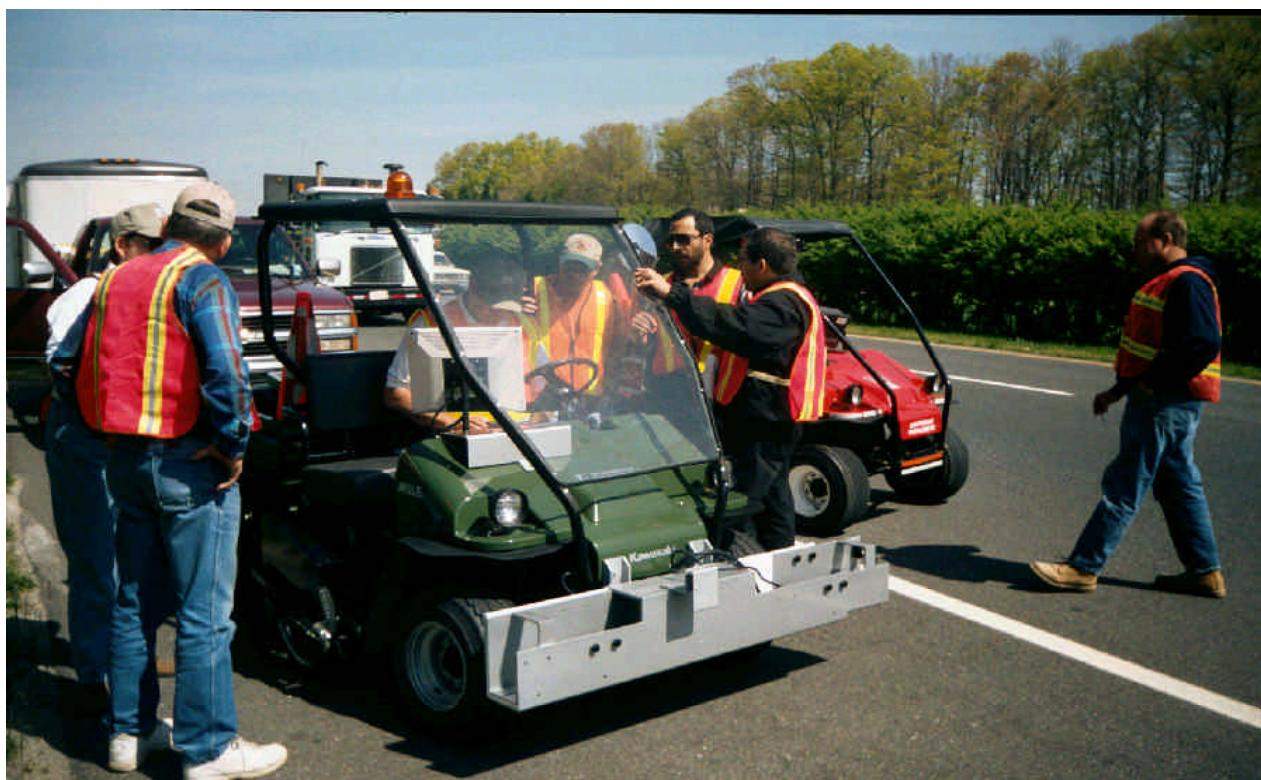
Figure 6. Phase II Testing (ICC Light Weight Profiler)
