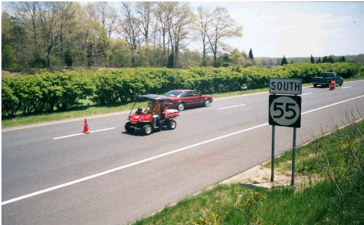
Figure 5. Phase II Testing (K. J. Law Light Weight Profiler)
