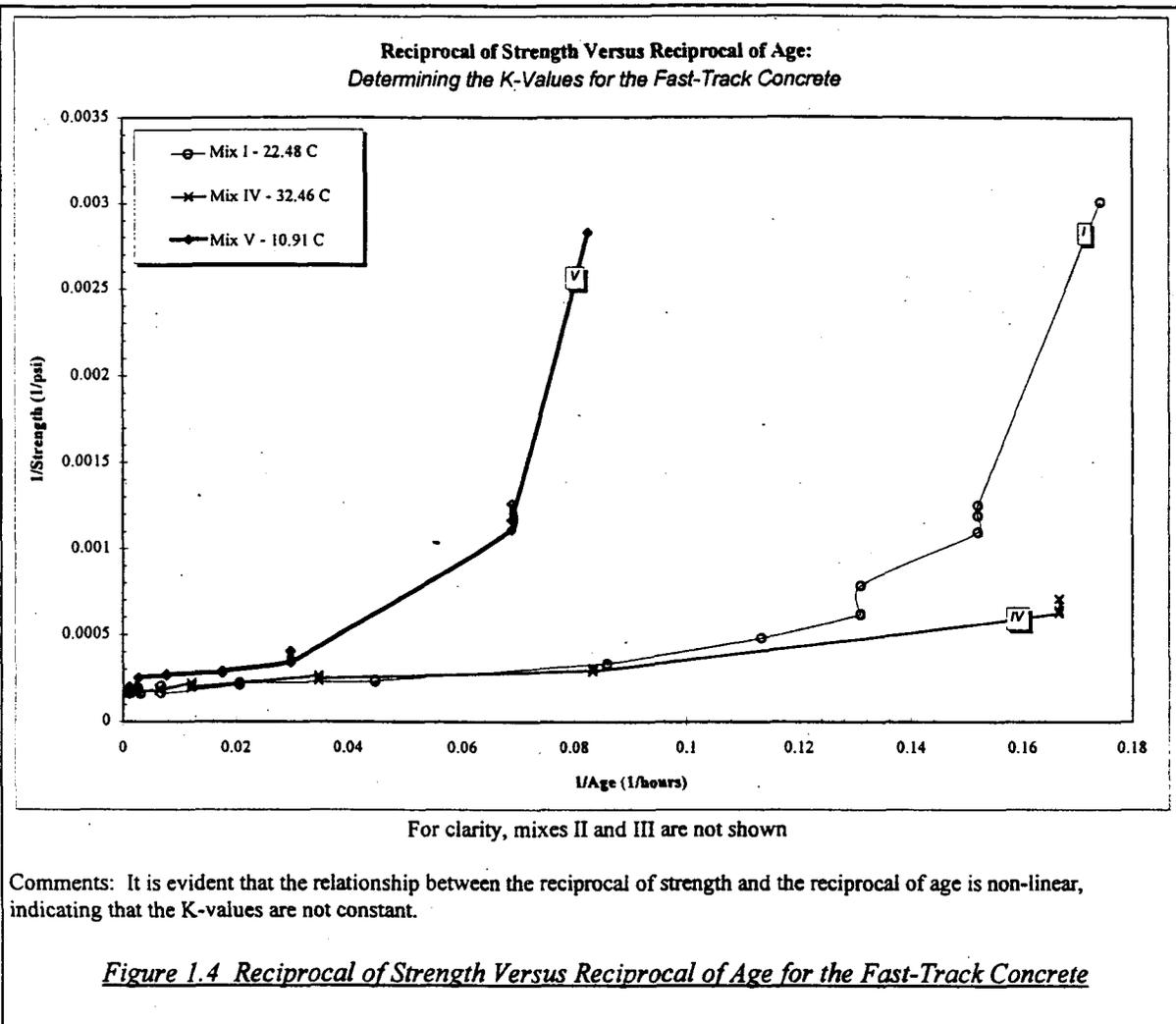
From Figure 1.4, it is evident that the K-values are not constant for the fast-track concrete, over time; i.e., the curves are not straight lines. The curves only approach linearity for times exceeding 12 hours at high temperatures, and 48 hours at very lower temperatures.
