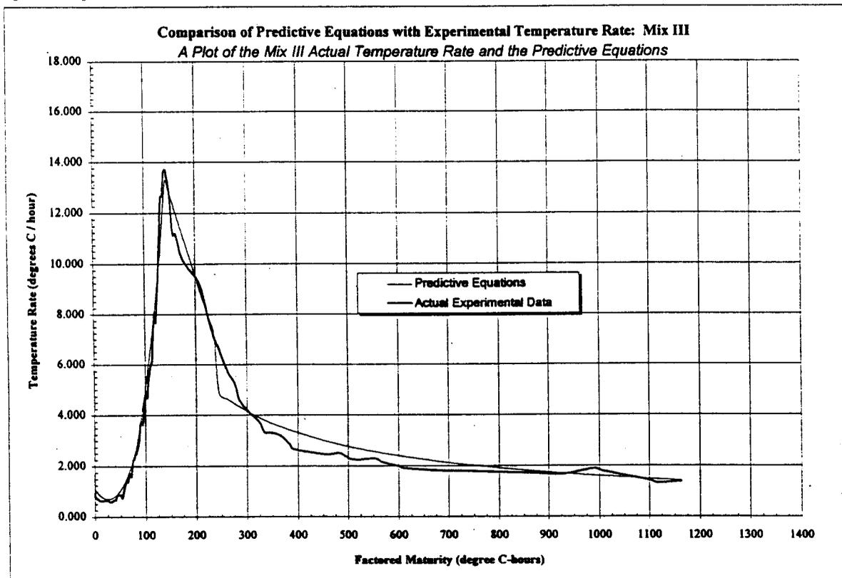
Figure 2.11 Comparison of Predictive Equations with Experimental Temperature Rate: Mix III
