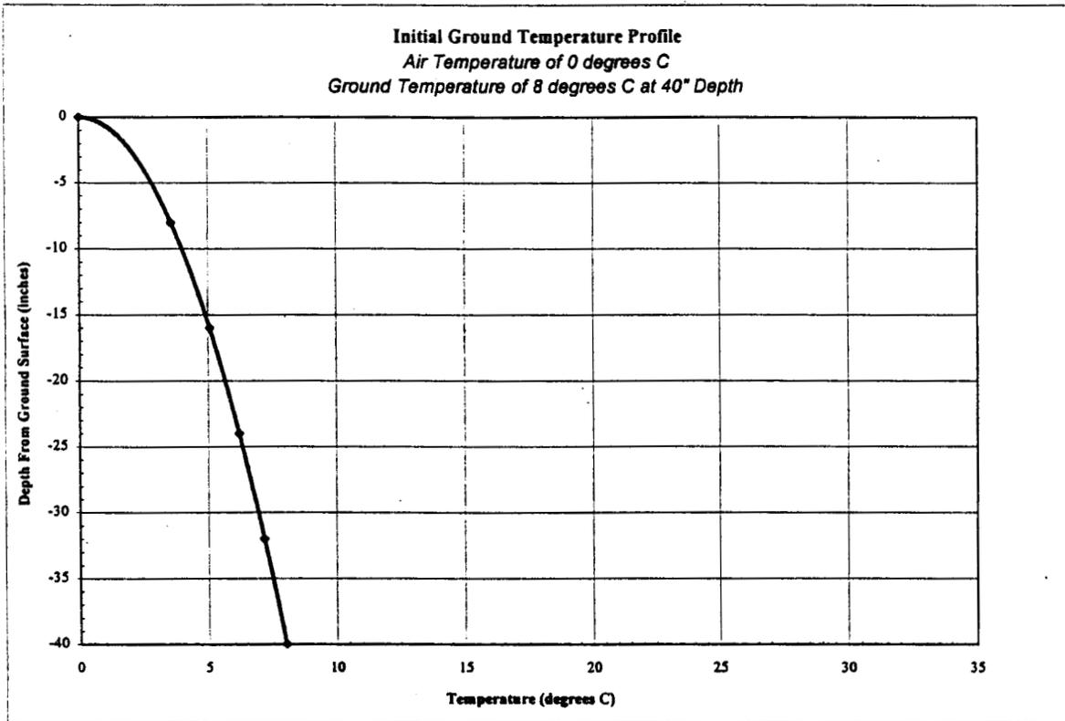
**Figure 3.2 - Computer Simulation's Initial Ground Temperature Profile**
