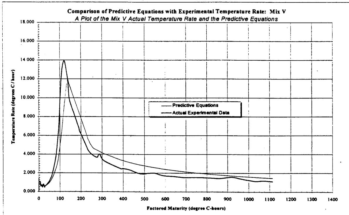
**Figure 2.13 Comparison of Predictive Equations with Experimental Temperature Rate: Mix V**
