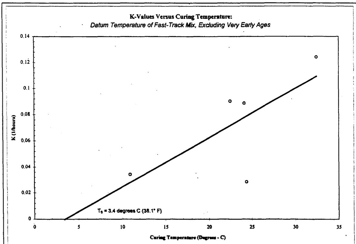
By excluding the very early age data points, the computed datum temperature reflects the datum at later ages, approaching infinity. This datum is only applicable after about 12 hours elapsed. With the K-values determined, the long-term datum temperature can be estimated. A best-fit line is made for the five K-values, previously computed. From the best-fit line, the datum temperature is 3.4° C (38.1° F)
