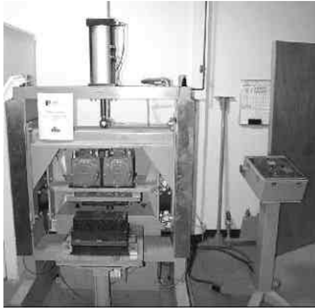
Figure 5: Asphalt Vibratory Compactor at RAPL
