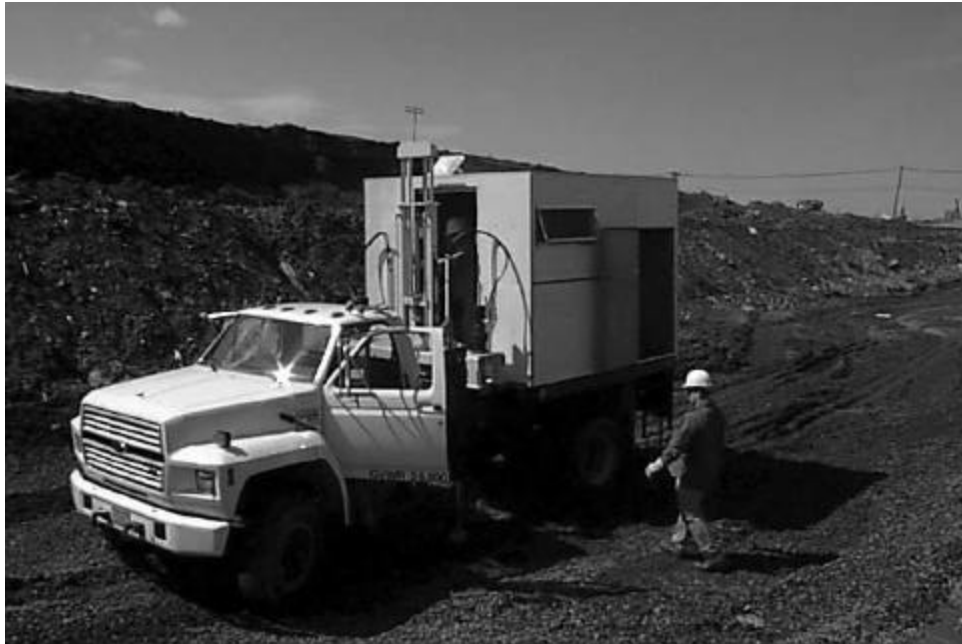
Figure 2 – Rutgers University Geotechnical Group's Cone Penetrometer Truck
