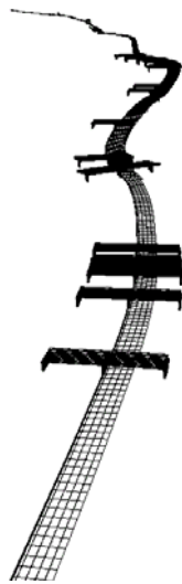
a) Portion of I-280 model showing bridge overpass structures positioned relative to roadway
