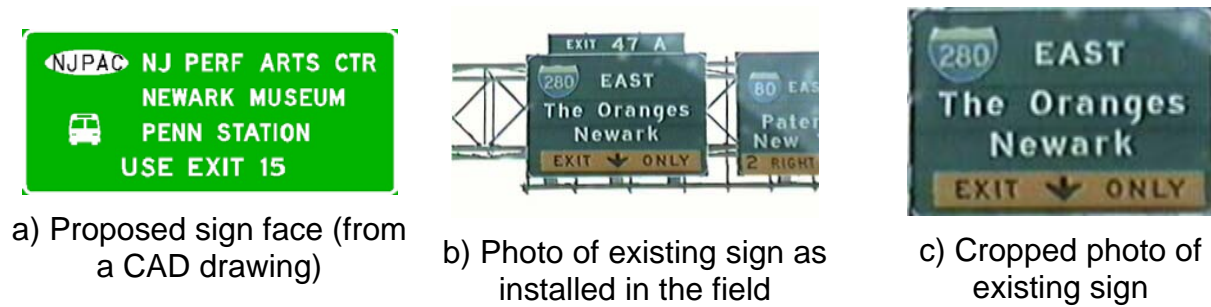
Figure 6. Use of raster image storage to represent both proposed signage and existing signage.
