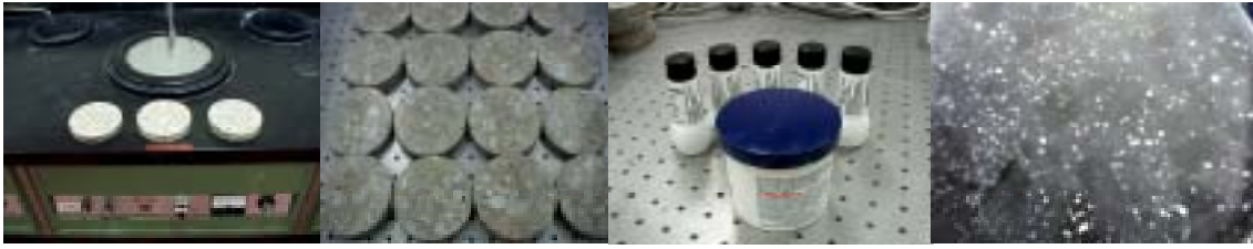
Figure 9. Concrete slice sample preparation. (From left to right: lapping machine, slice after polishing, painting materials, sample ready for test)
