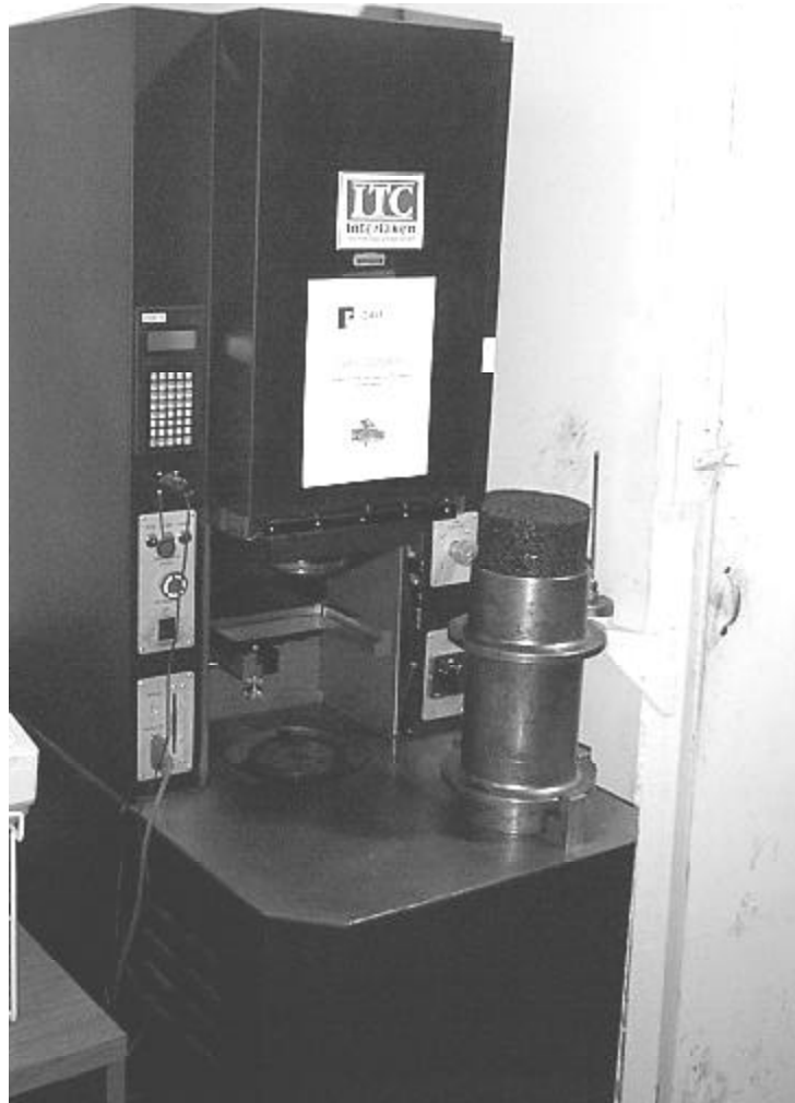
Figure 3 – Superpave Gyratory Compactor at RAPL
