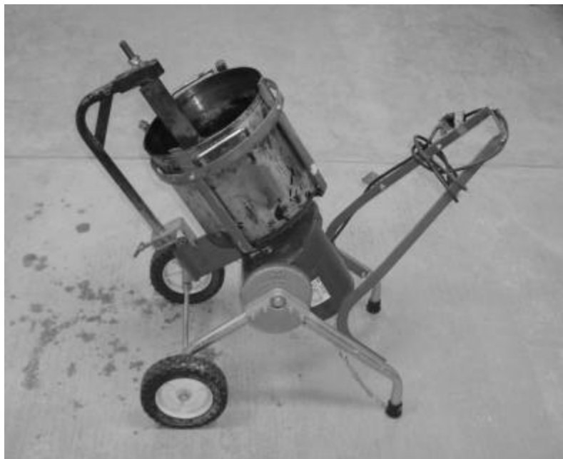
Figure 10 - Rotating 5-gallon Stainless Steel Mixing Bucket
