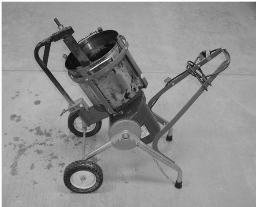
Figure 16 - Rotating 5-gallon Stainless Steel Mixing Bucket
