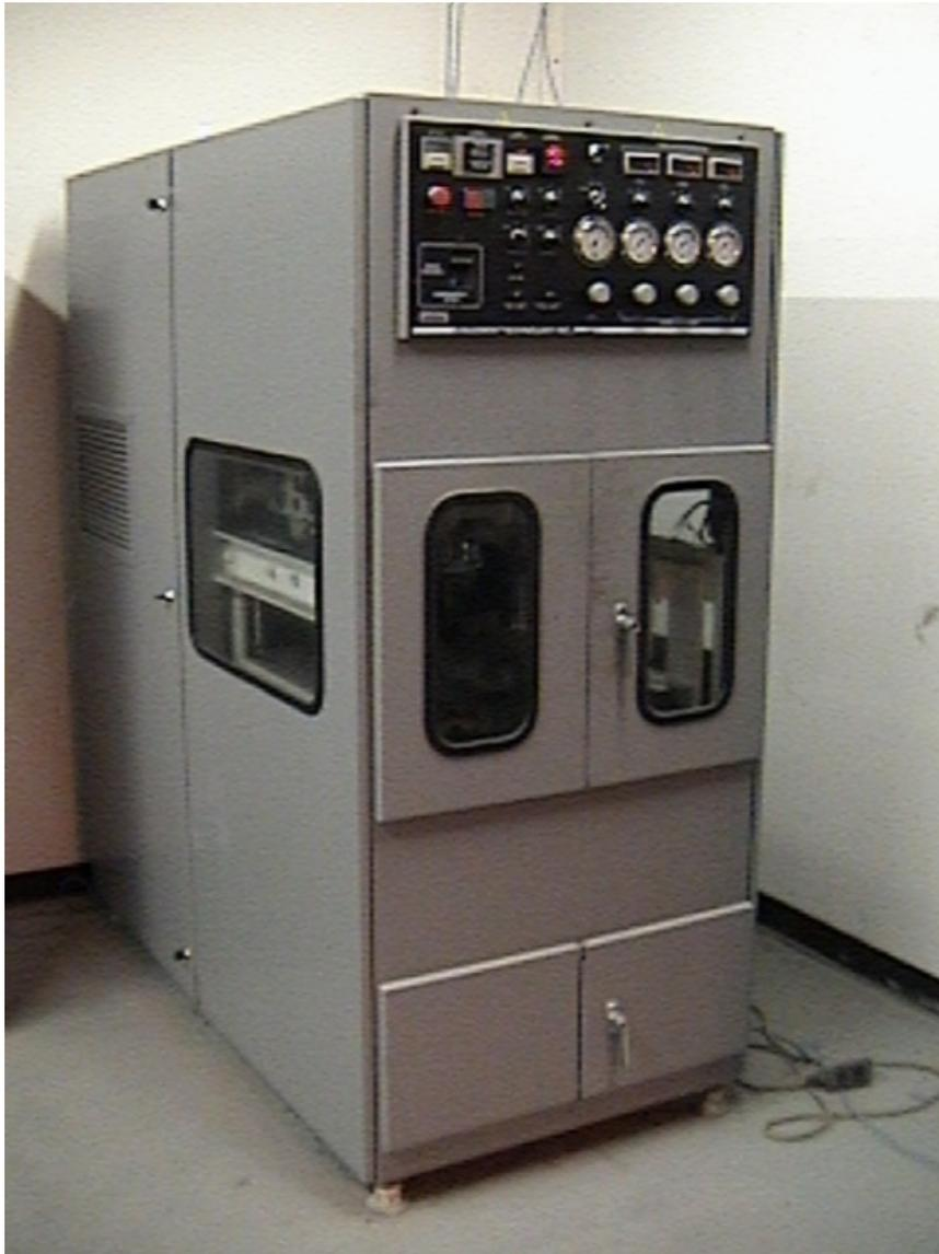
Figure 12 – Asphalt Pavement Analyzer
