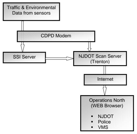
Figure 5. Schematic representation of the working of the deployed weather information system on the Wanaque Bridge
