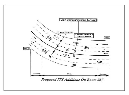
Figure 2. Schematic of the Proposed Weather System for Wanaque Bridge
