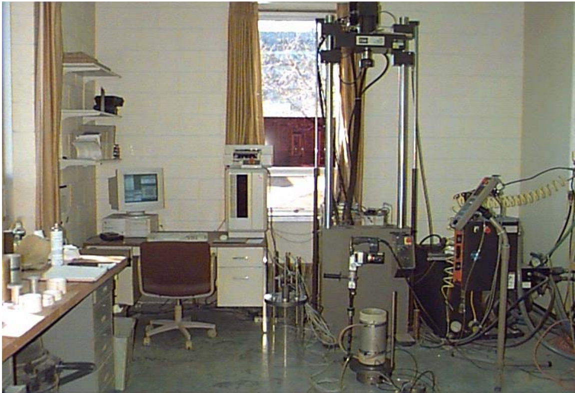
Figure 25 – Test Set-up Used to Conduct Resilient Modulus Testing
