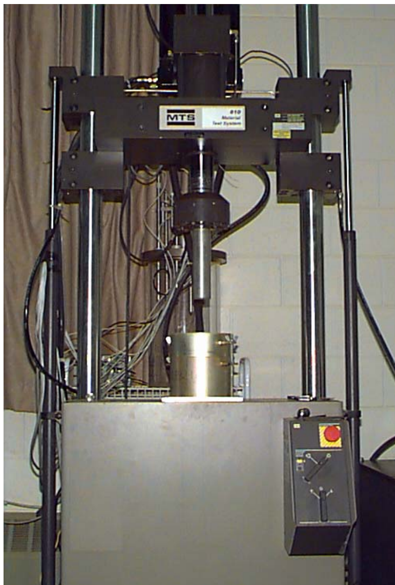
Figure 15 – Testing Set-up Used for the CBR Testing
