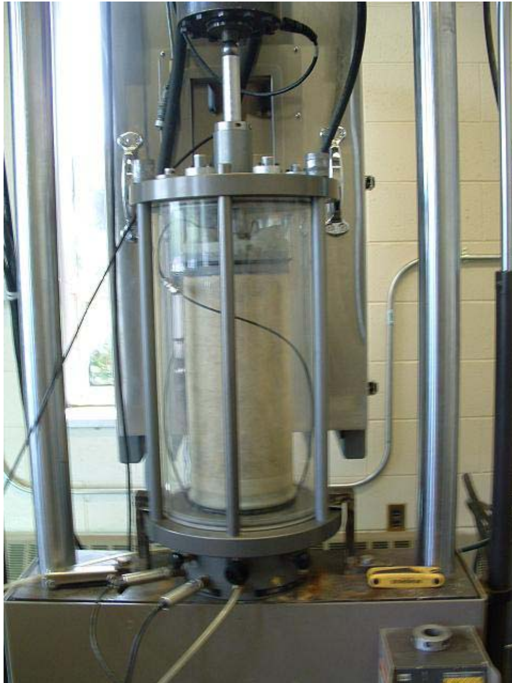
Figure 23 – Test Set-up Used for Triaxial (Static and Cyclic) and Resilient Modulus Testing
