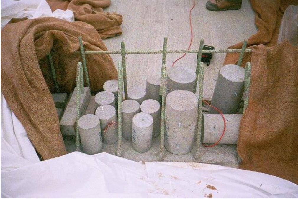
Figure 14. Field matched-cured specimen
