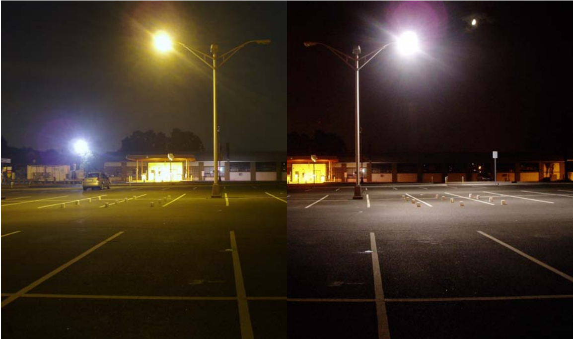
Figure 64: Positive and Null contrast test with HPS and white light source- Three pole spacing
