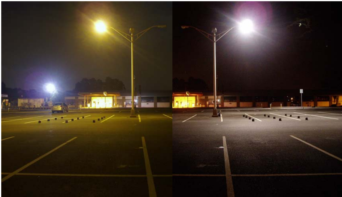
Figure 63: Negative contrast test with HPS and white light source- Three pole spacing
