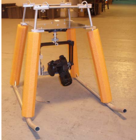
Figure 19: Custom mount and vibration damping undercarriage.
