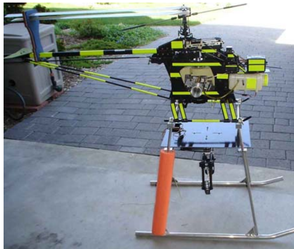
Figure 20: Helicopter with final vibration damping undercarriage.
