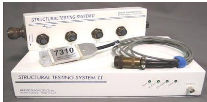
Figure 13. Structural testing system by Bridge Diagnostics Inc.
