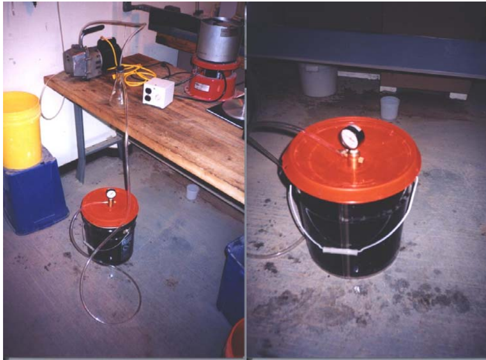
Figure 19 Photograph of vacuum container with vacuum pump and gage.
