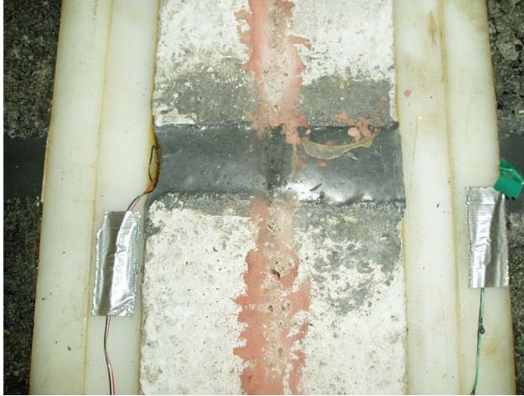
Figure 36 Rutting of concrete sample after 100,000 cycles.
