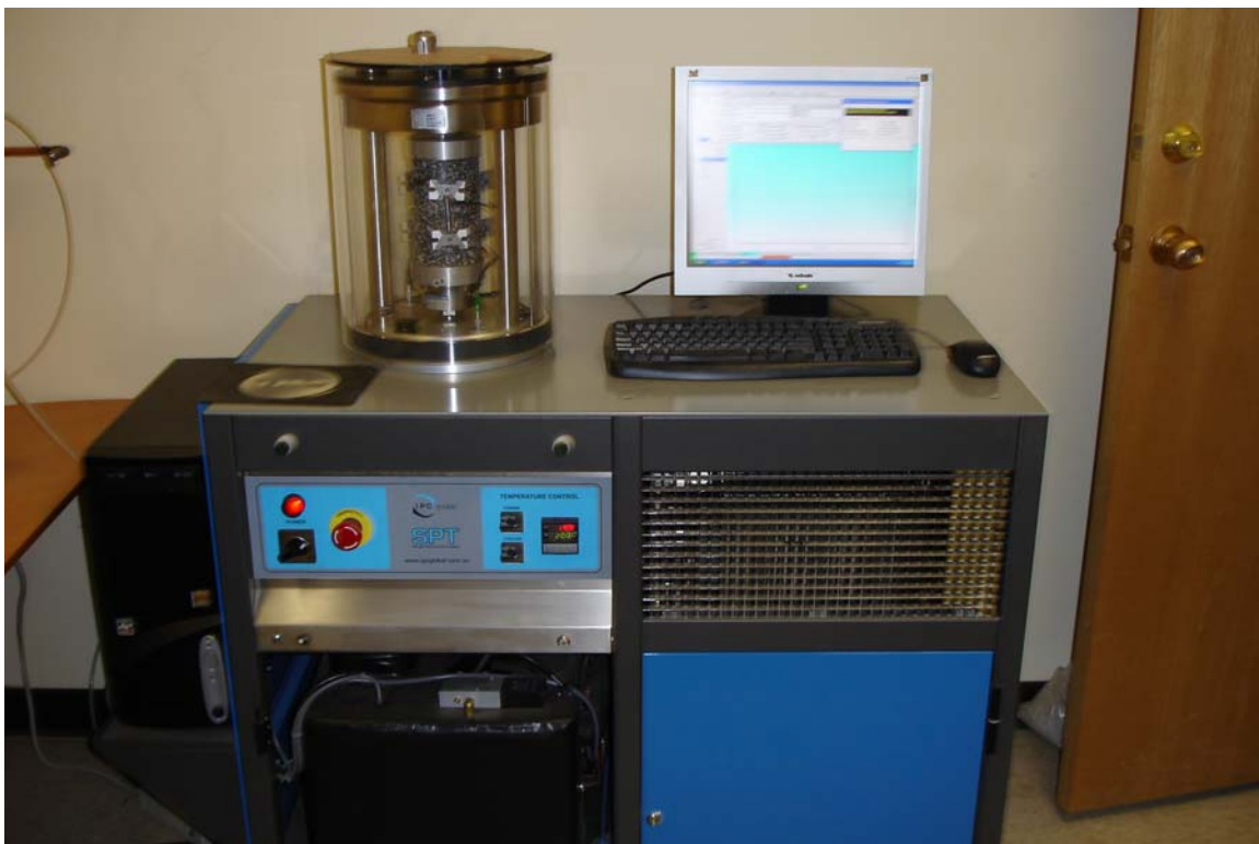
Figure 22 – Dynamic Modulus Test Device
