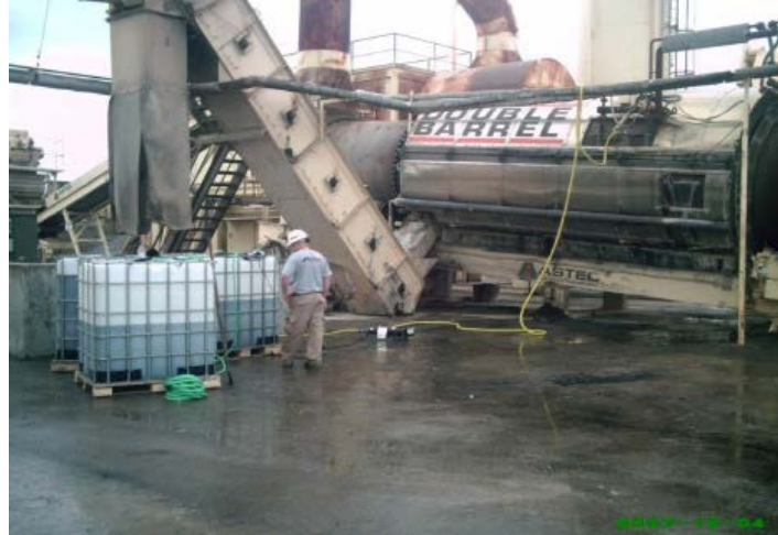
Figure 2. Evotherm Added to Drum (85% Water; 15% “Chemical Package”)
