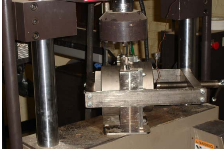
Figure 11. NCAT Bond Strength Test Device (Picture of Rutgers U. Unit)
