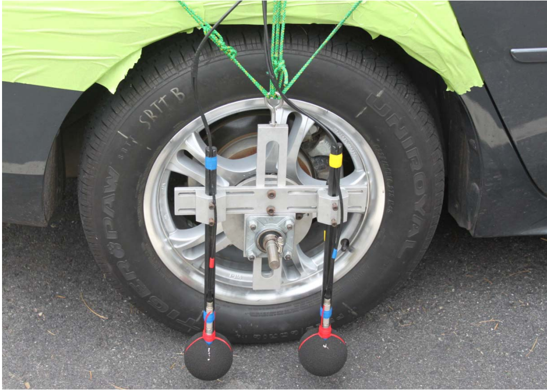
Figure 1: Sound Intensity Testing Apparatus
