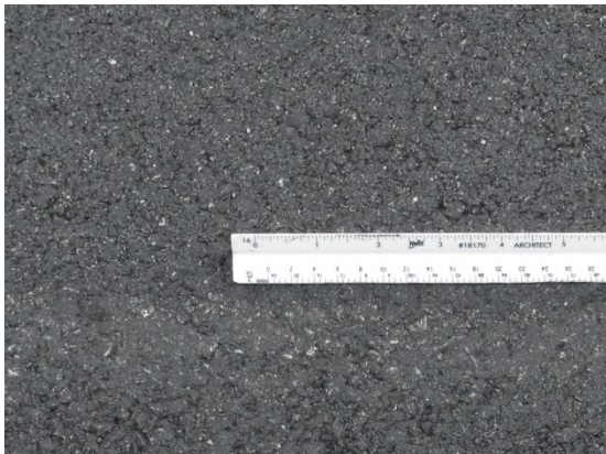
Figure 16: I-495 S 9.5mm Superpave + 2% latex
