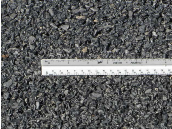
Figure 15: Rt. 2 19mm Superpave
