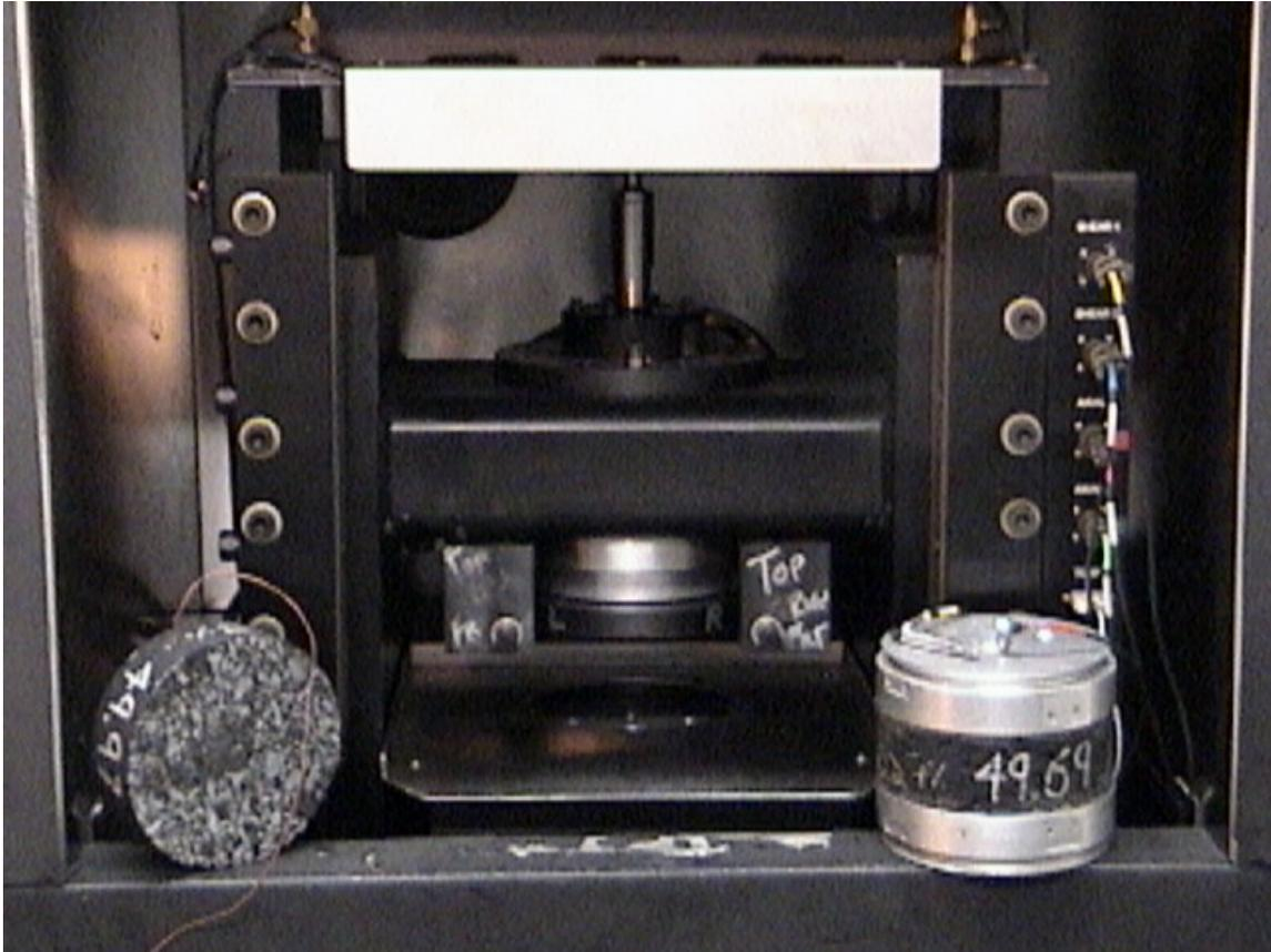
Figure 4.4 – Superpave Shear Tester (SST)
