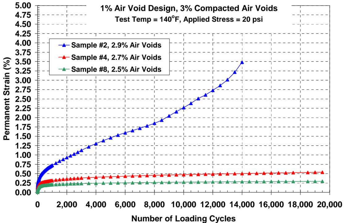
Figure 3.3 – Permanent Deformation Plots of 1% Air Void Design and 3% Air Void Compacted
