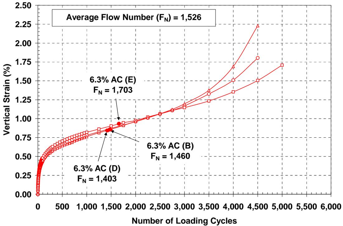
Figure 1.4 – Repeated Load Permanent Deformation Test Results for I-5 with 6.3% AC
