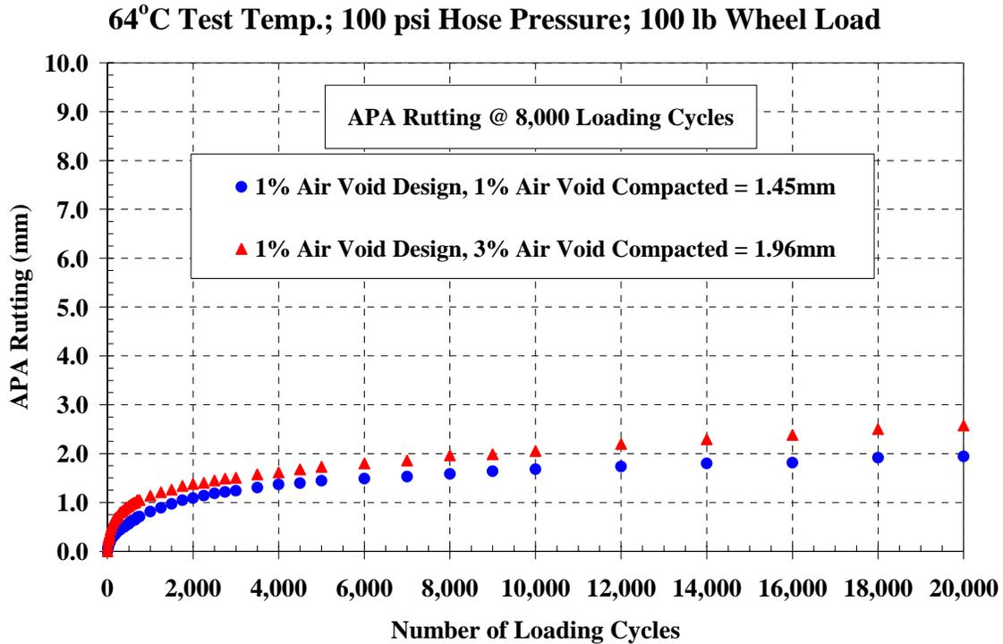
Figure 3.4 – Asphalt Pavement Analyzer Test Results for Rosphalt 50 Samples
