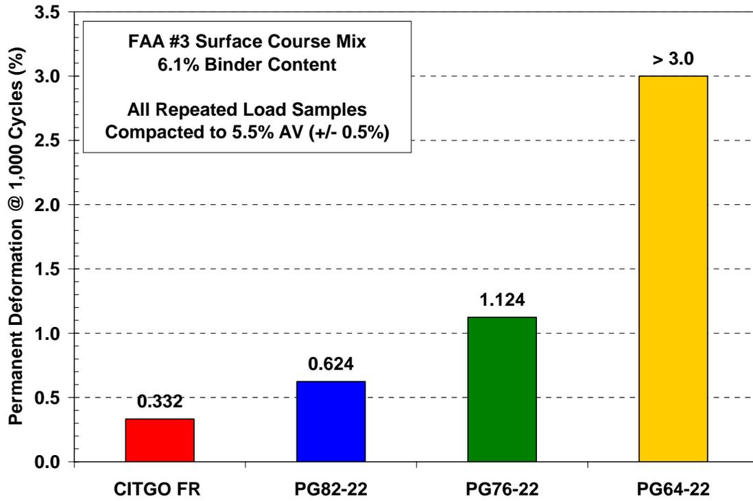
Figure 5.13 - Summary of Permanent Deformation @ 1,000 Loading Cycles from Repeated Load Permanent Deformation Testing (Higher Permanent Deformation, Higher Rutting Potential)
