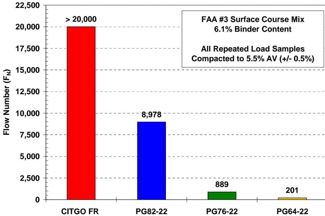
Figure 5.11 – Summary of Flow Number Results from Repeated Load Permanent Deformation Testing (Higher F<sub>N</sub>, Lower Rutting Potential)
