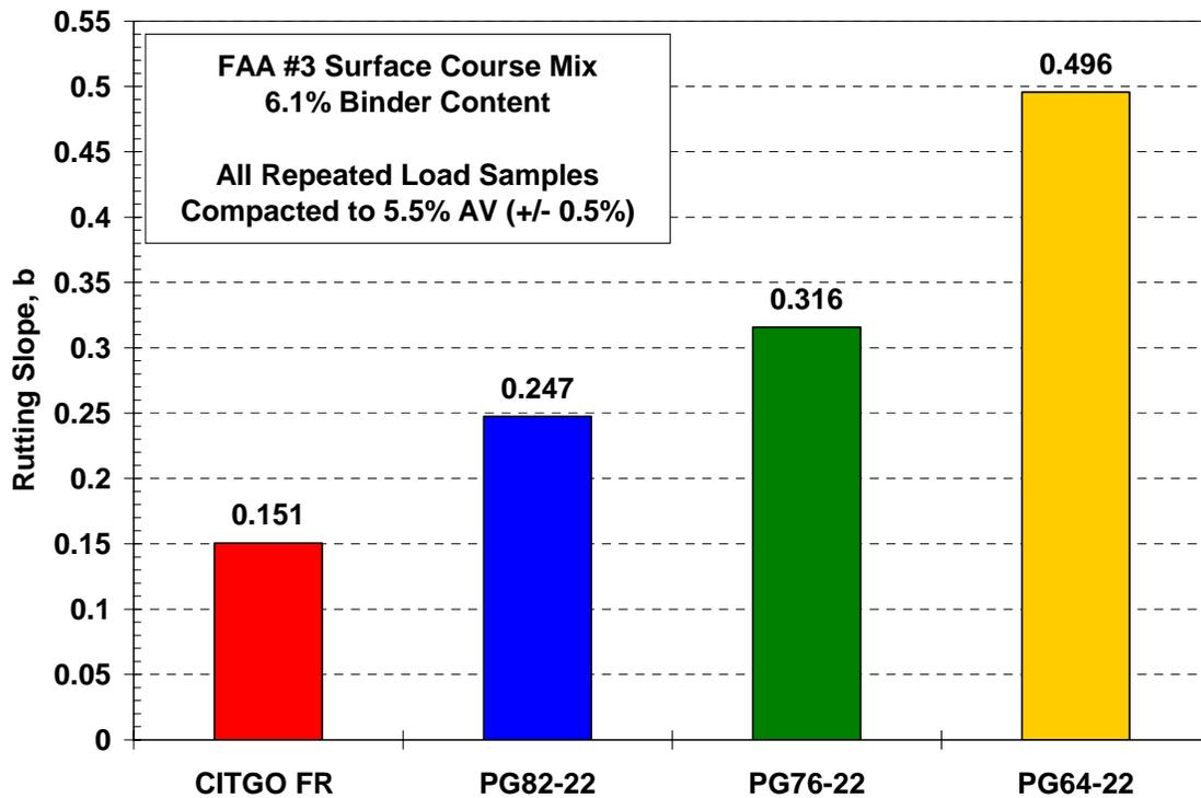
Figure 5.12 – Summary of Rutting Slope, b, Results from Repeated Load Permanent Deformation Testing (Higher b, Higher Rutting Potential)
