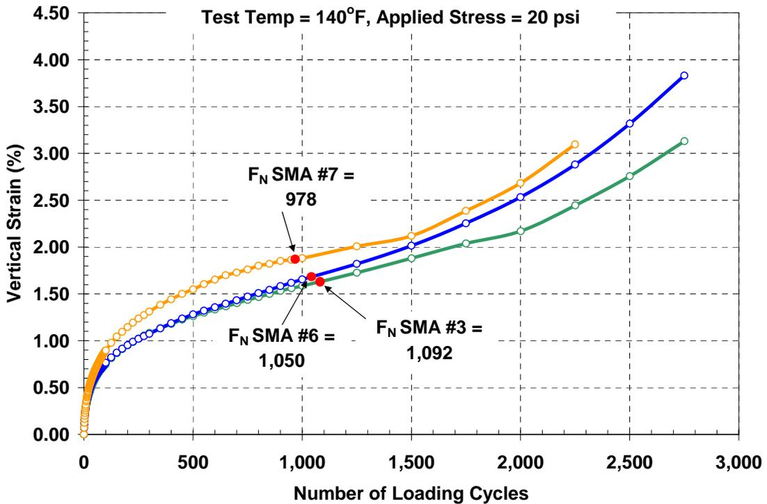
Figure 1.2 – Repeated Load Permanent Deformation Test Results for Port Authority SMA Mix
