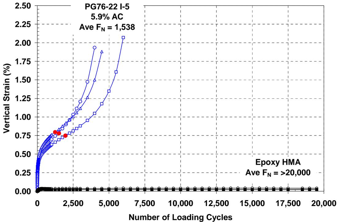
Figure 2.3 – Comparison of Repeated Load Permanent Deformation Test Results for the PANYNJ Epoxy HMA and PG76-22 I-5 Mix (5.9% AC)
