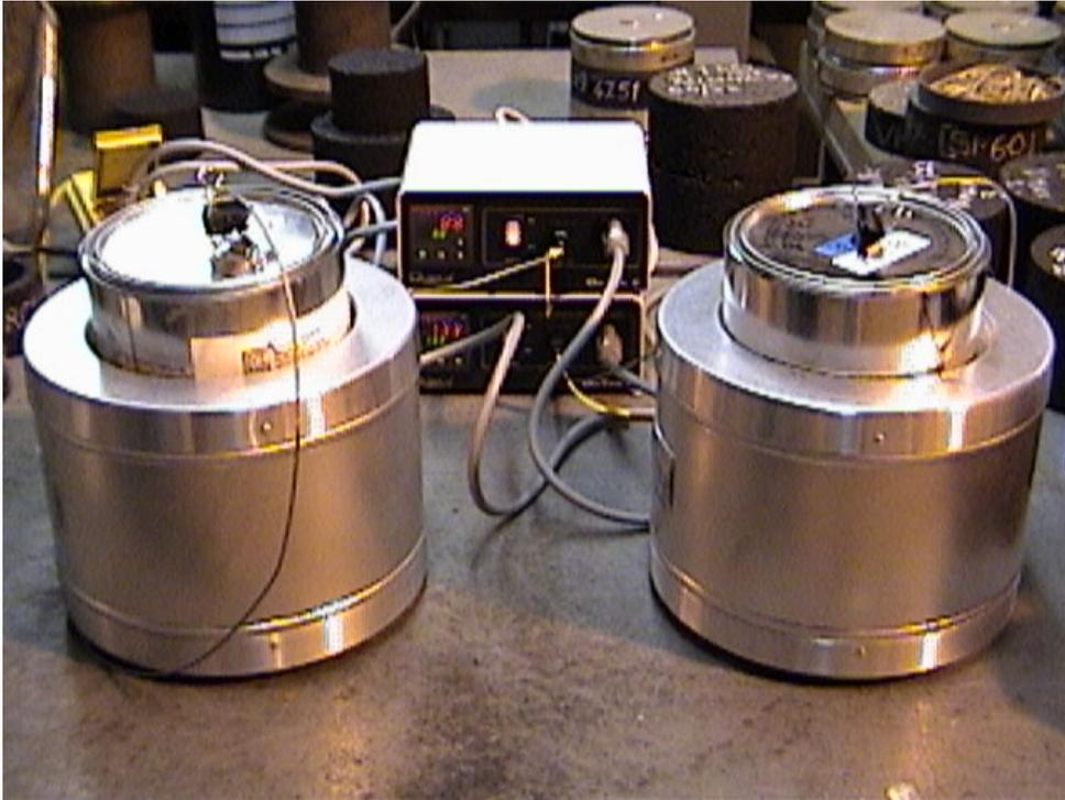
Figure 2.1 – Gallon Can Heaters Used for Blending and Mixing the Epoxy Asphalt Binder
