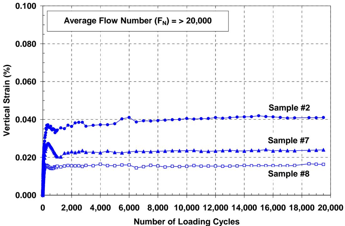
Figure 2.2 – Repeated Load Permanent Deformation Test Results for the Port Authority Epoxy HMA Mix
