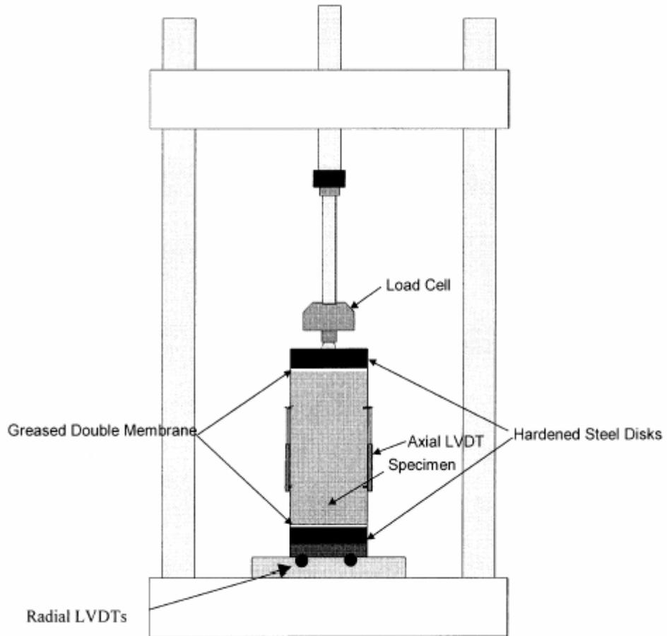
Figure 1. Schematic of repeated load permanent deformation test.
