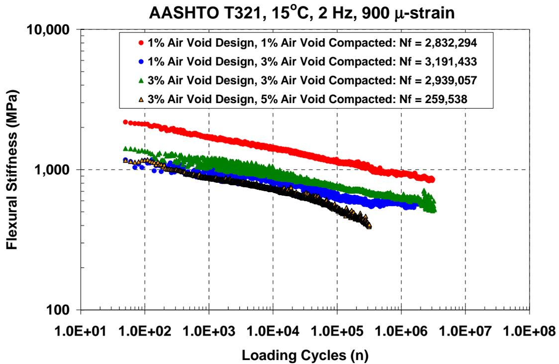
Figure 3.1 – Flexural Beam Fatigue Test Results for the Rosphalt 50 Material
