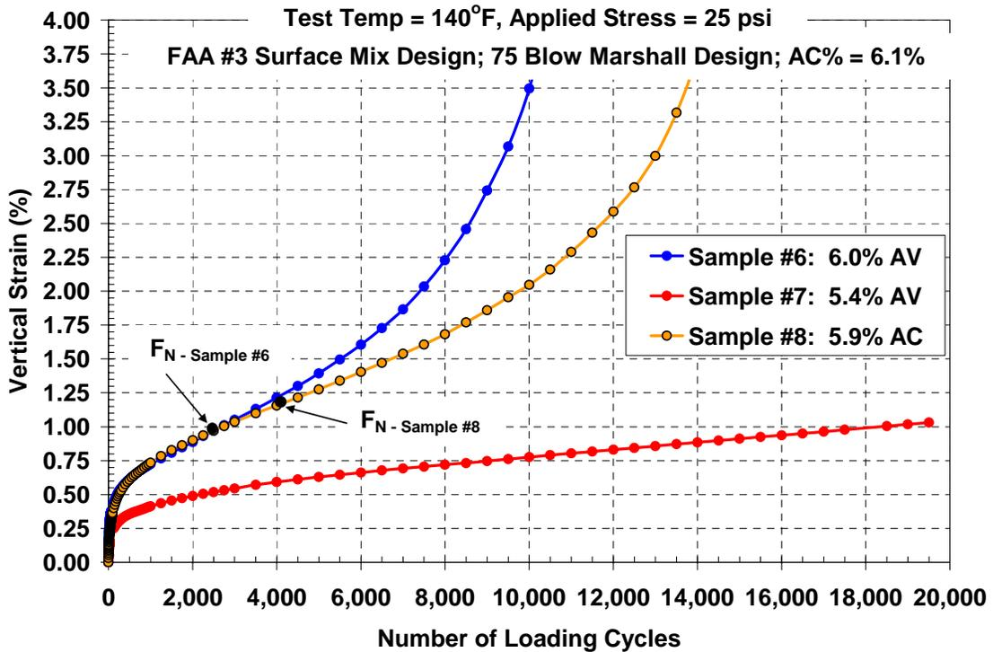
Figure 5.8 – FAA #3 Surface Course Mix with PG82-22 Asphalt Binder (CITGO Asphalt)
