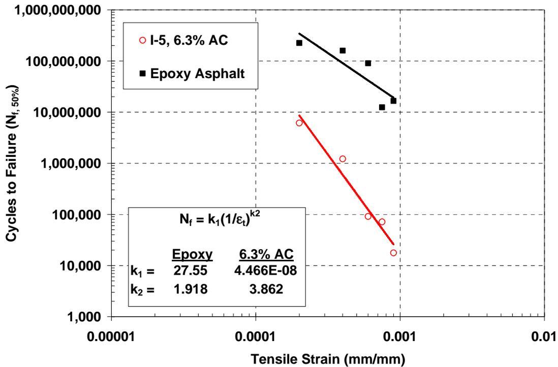
Figure 2.4 – Fatigue Properties of Epoxy Asphalt and PG76-22 I-5 Samples (6.3% AC)
