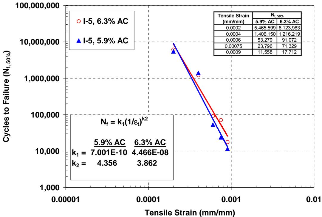
Figure 1.5 – Fatigue Properties of I-5 Samples with 5.9% and 6.3% AC
