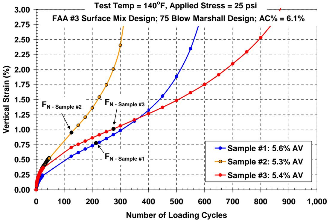
Figure 5.10 – FAA #3 Surface Course Mix with PG64-22 Asphalt Binder (CITGO Asphalt)
