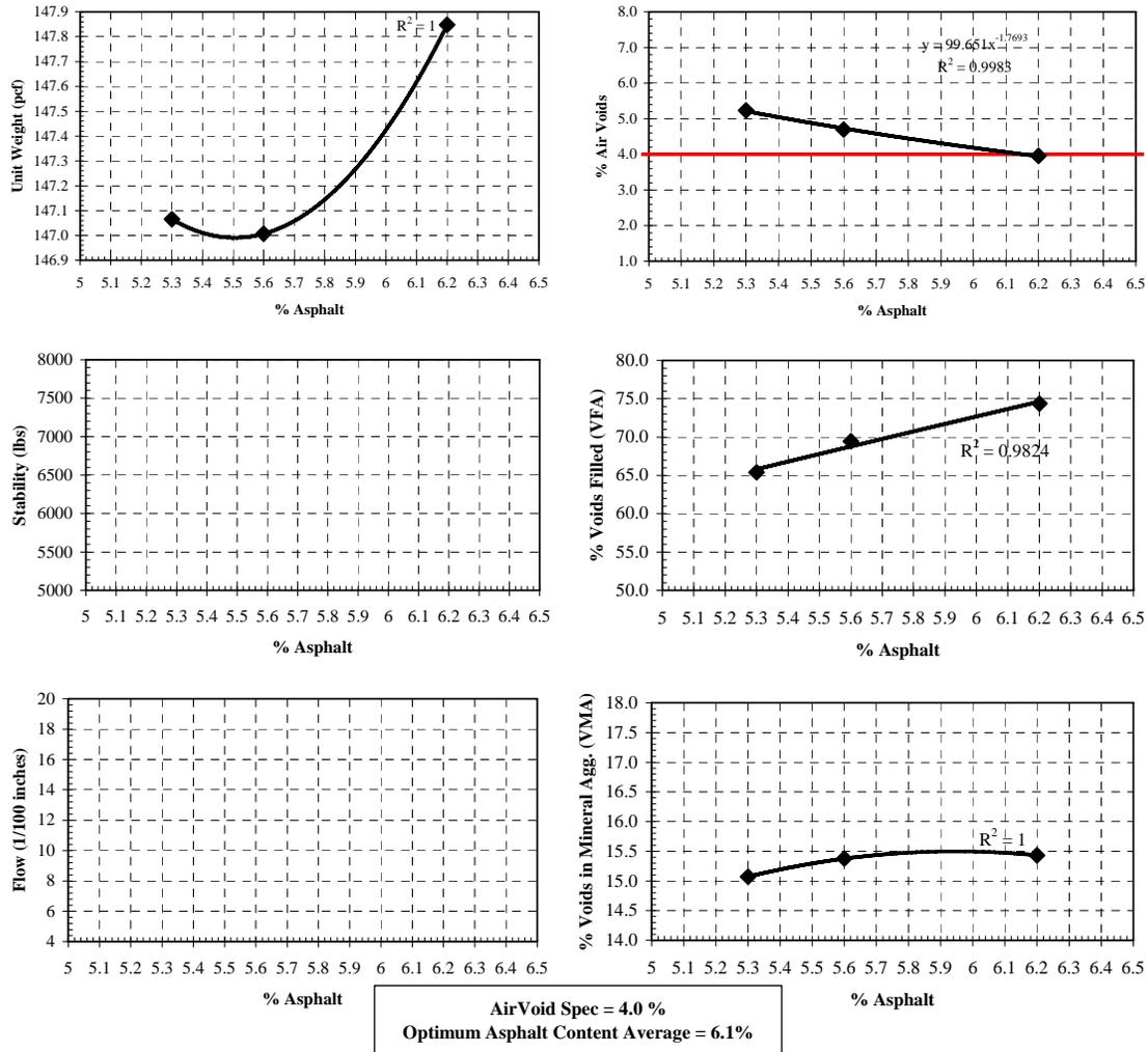
Figure 5.2 – 75 Blow Marshall Design Results for FAA #3 Surface Course Mix
