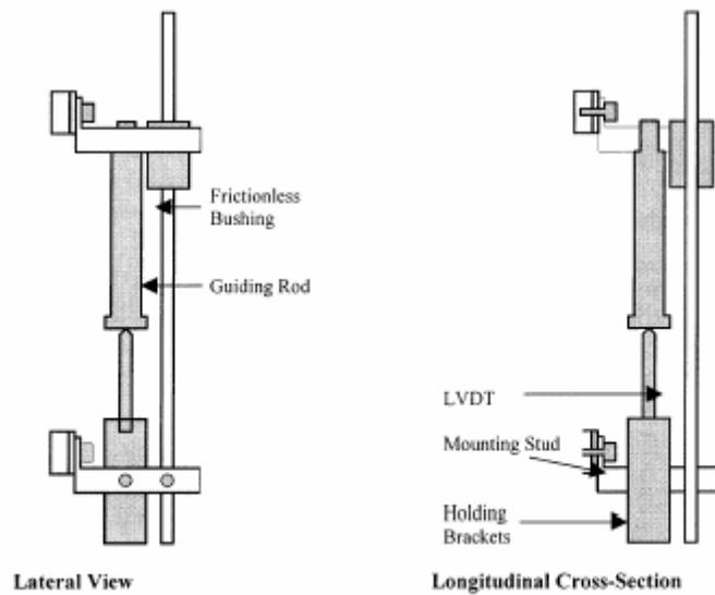
Figure 2. Axial LVDTs instrumentation.
