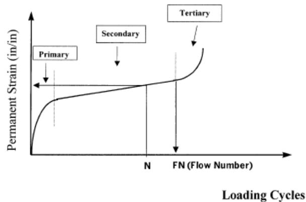
Figure 5.5 – Example of Flow Number During Repeated Load Test
