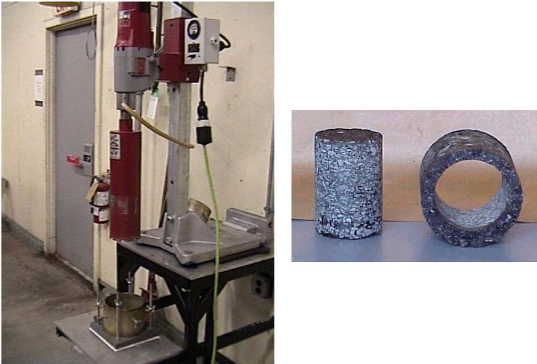
Figure 5.3 – Sample Preparation for Repeated Load Using the SPT Set-up
