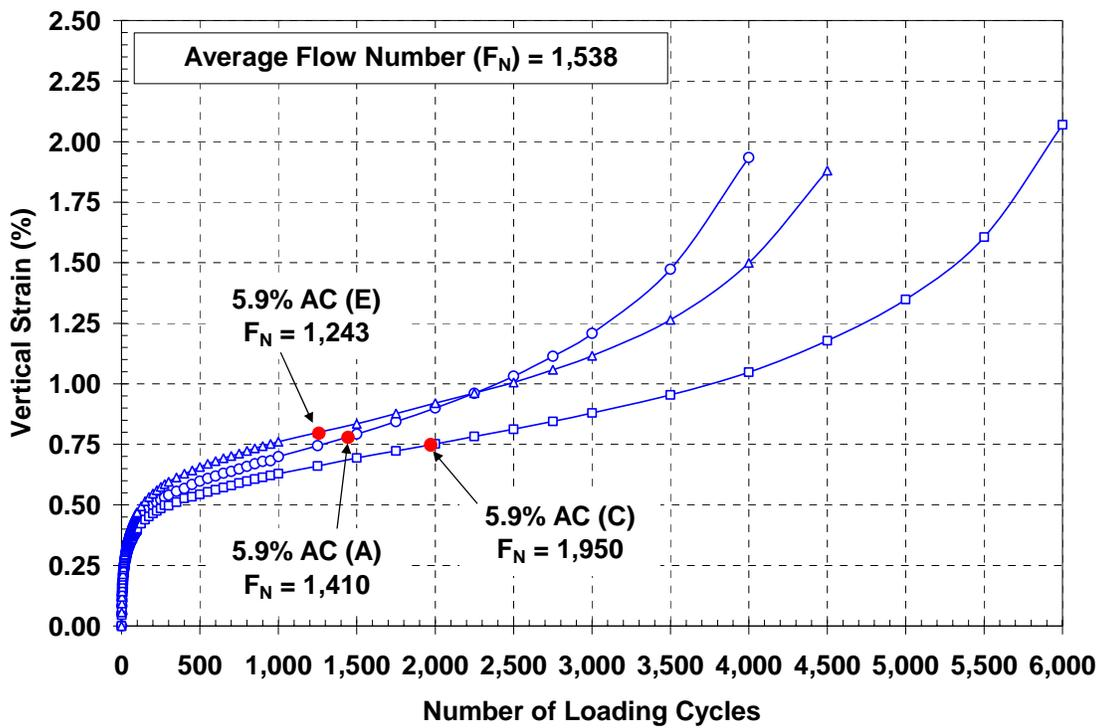
Figure 1.3 – Repeated Load Permanent Deformation Test Results for I-5 with 5.9% AC
