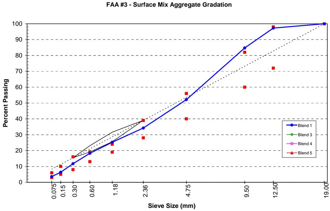
Figure 5.1 – Aggregate Gradation of FAA #3 Surface Course Mix Used in Study (Mt. Hope Aggregates)
