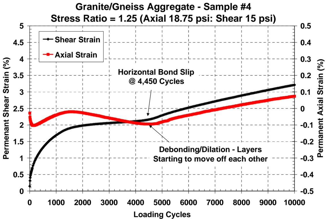
Figure 4.6 – Granite/Gneiss Core #4
