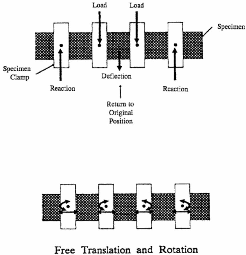
**Figure 1. Load and Freedom Characteristics of Fatigue Test Apparatus**
