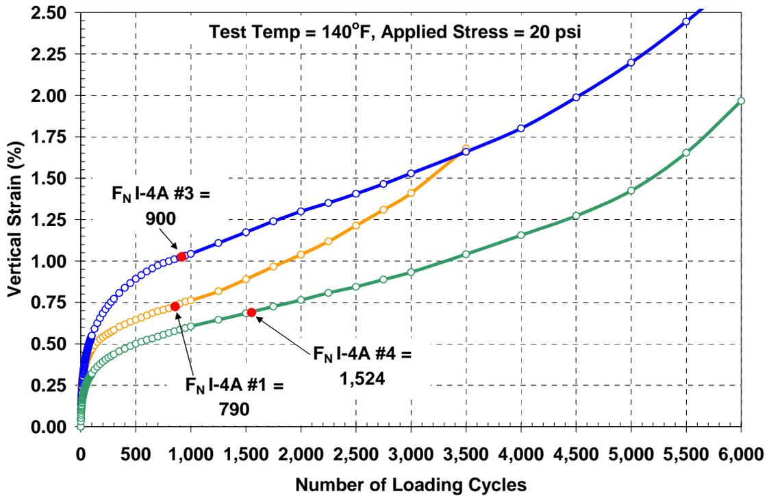
Figure 1.1 – Repeated Load Permanent Deformation Test Results for the Port Authority I-4A HMA Mix
