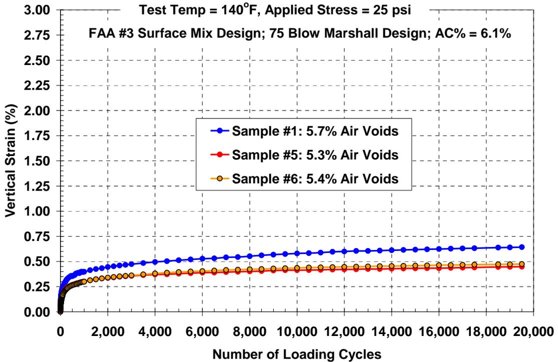
Figure 5.7 – FAA #3 Surface Course Mix with CITGO Fuel Resistant Asphalt Binder
