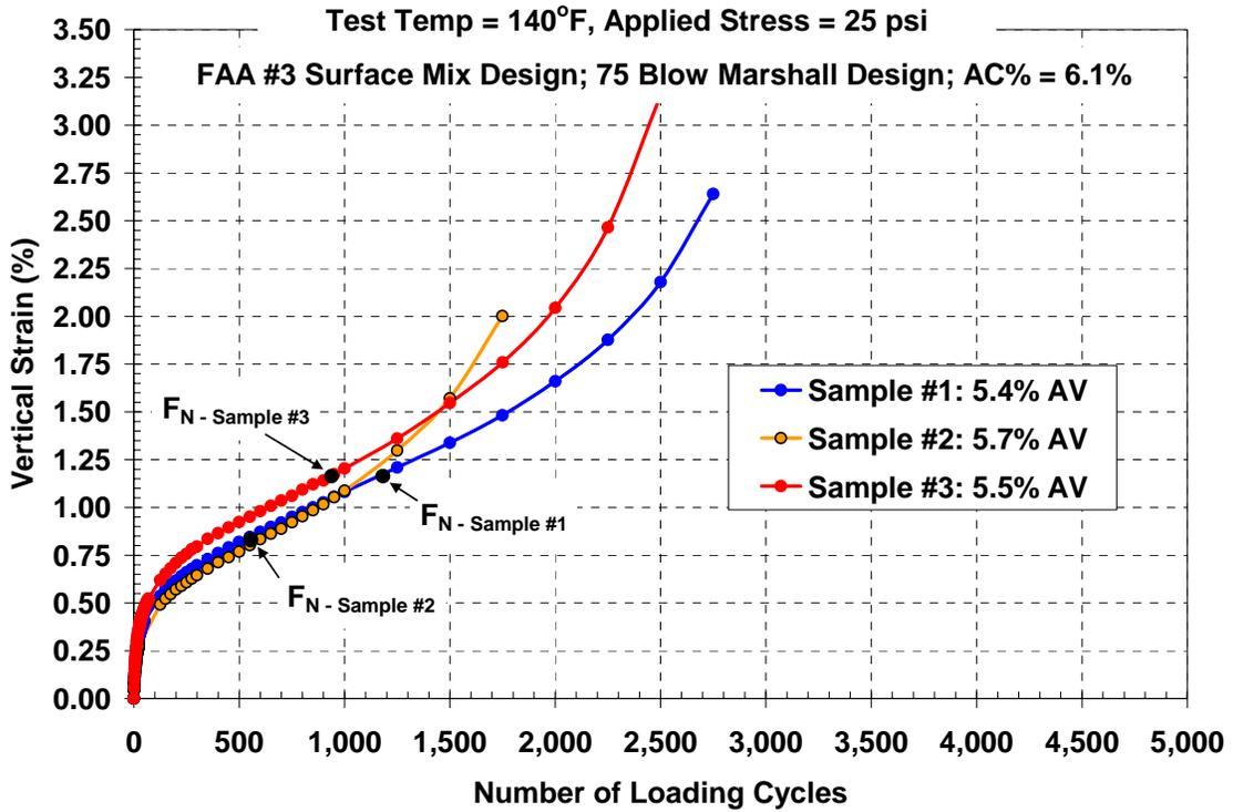
Figure 5.9 – FAA #3 Surface Course Mix with PG76-22 Asphalt Binder (CITGO Asphalt)
