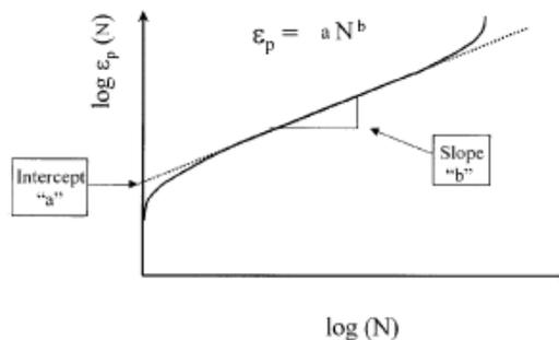
Figure 5.6 – Example of Slope, b, During the Repeated Load Test
