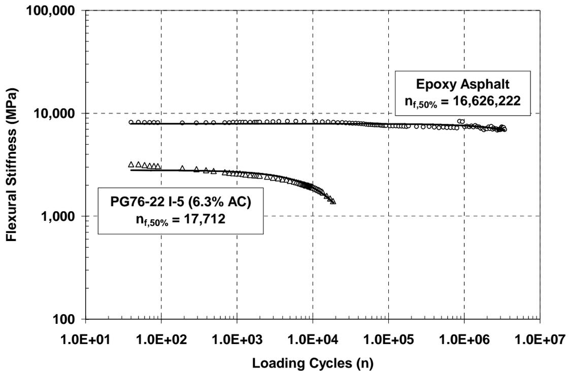
Figure 2.5 – Fatigue Life of Epoxy Asphalt and PG76-22 I-5 (6.3% AC) at 900 Micro-strains
