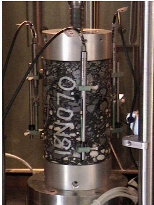
Figure 5.4 – Instrumented Simple Performance Test Specimen
