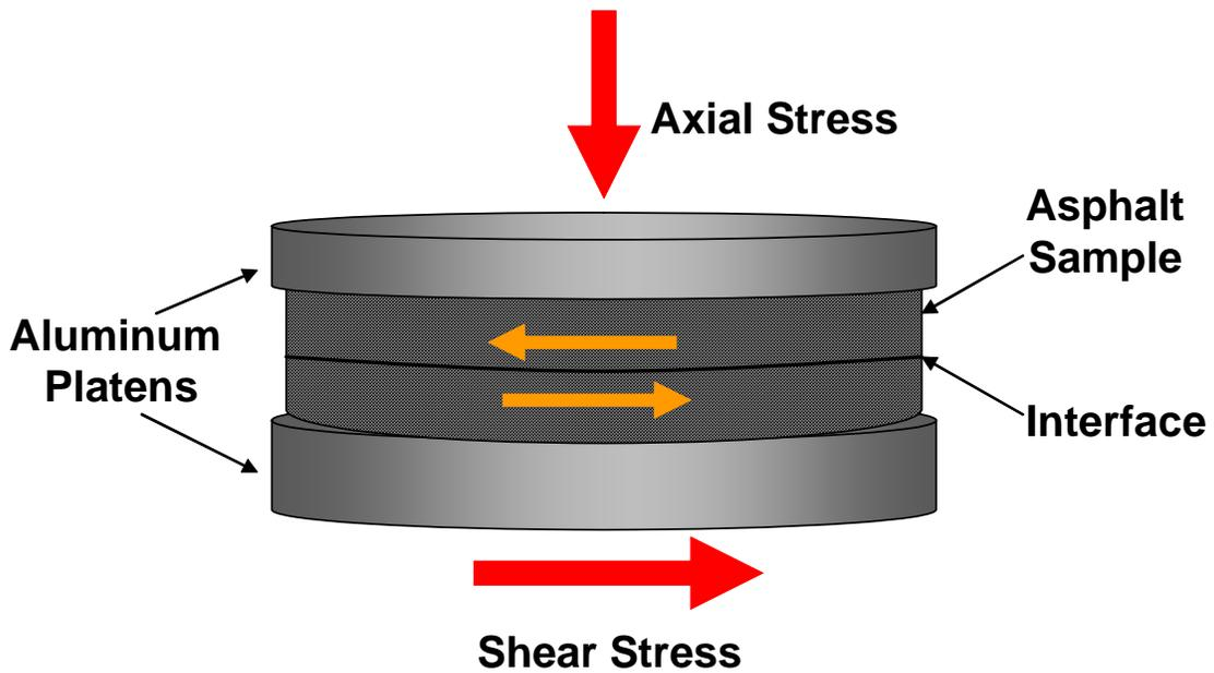
Figure 4.3 – Comparison of Field Stress and Laboratory Applied Stress Conditions
