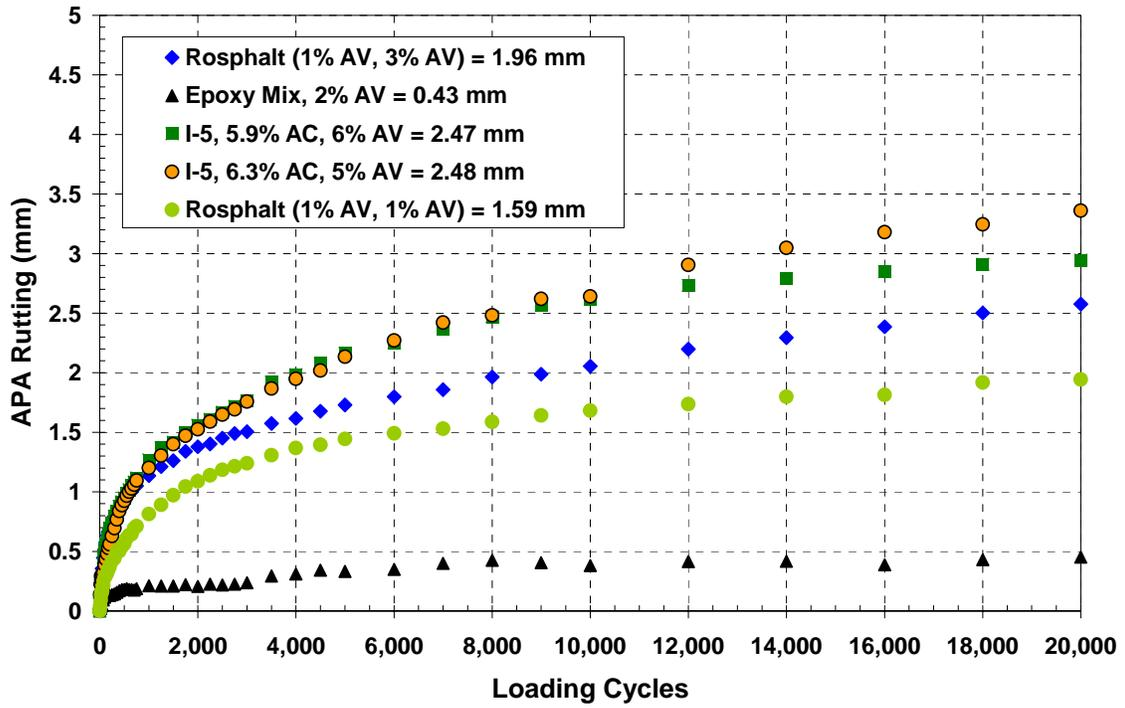
Figure 3.5 – Asphalt Pavement Analyzer Test Results
