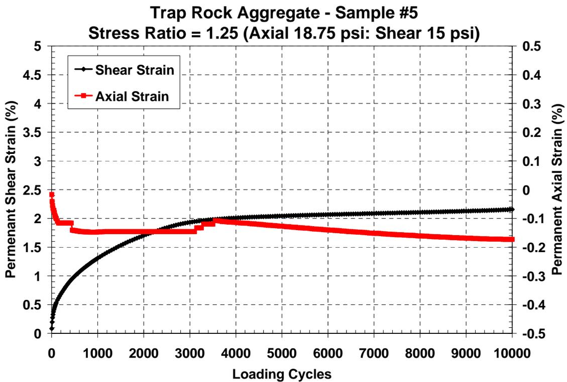
Figure 4.10 – Trap Rock Core #5
