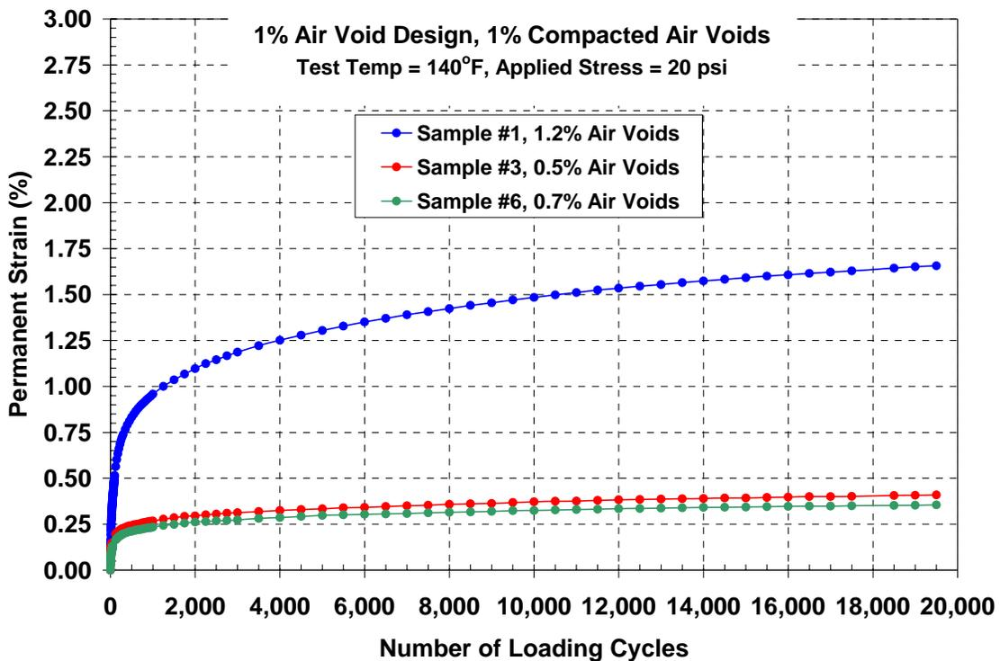
Figure 3.2 – Permanent Deformation Plots of 1% Air Void Design and 1% Air Void Compacted
