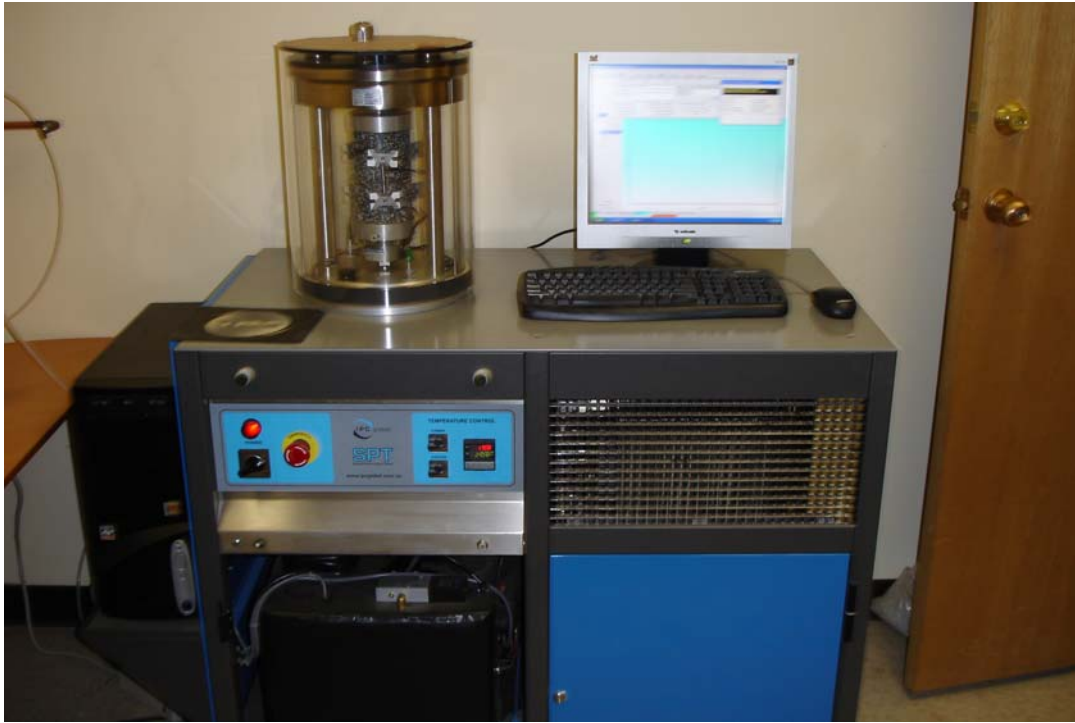
Figure 5 – Test Machine for Repeated Load and Dynamic Modulus Test
