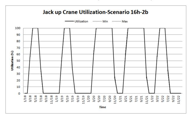
The average utilization for the Jack-up crane for the busy period is about 83%. This number can be broken down to 78% for half farm years and 87% for full farm years.
