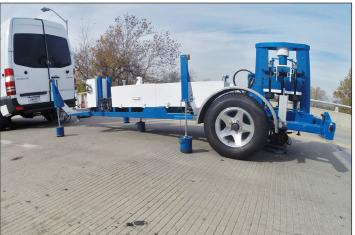
THMPER uses quantitative data to calculate a bridge's load capacity accurately, quickly, and with less traffic disruption.
