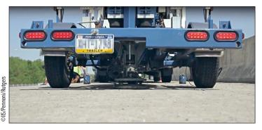
The THMPER™ impact trailer and sensors, rolling "control center," and custom software suite record the bridge's vibration response and process test data on the spot. Faster, cheaper, and with less traffic disruption than other methods, THMPER could revolutionize how bridge load ratings are determined.
