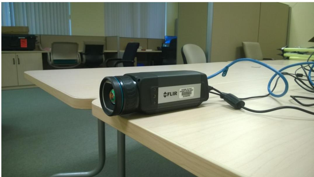
**Figure 9 The FLIR Infrared Camera**
