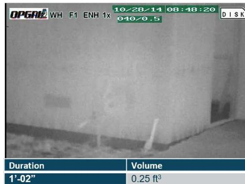
Figure 22 Successful Detection of Gas Leaks at 50 feet Distance
