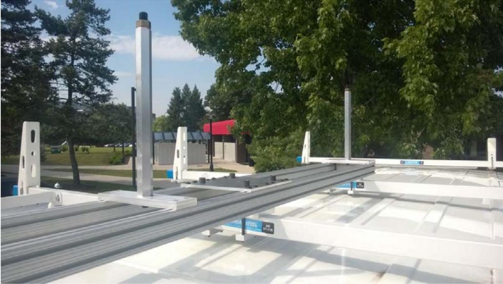
**Figure 5 The Installed Sensor Mounting Platform**
