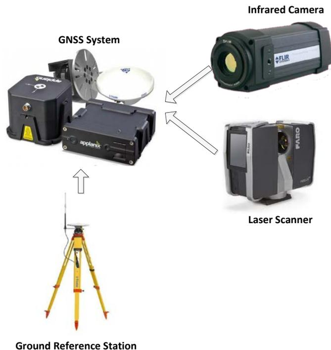
**Figure 4 The Mobile Mapping System Components**
