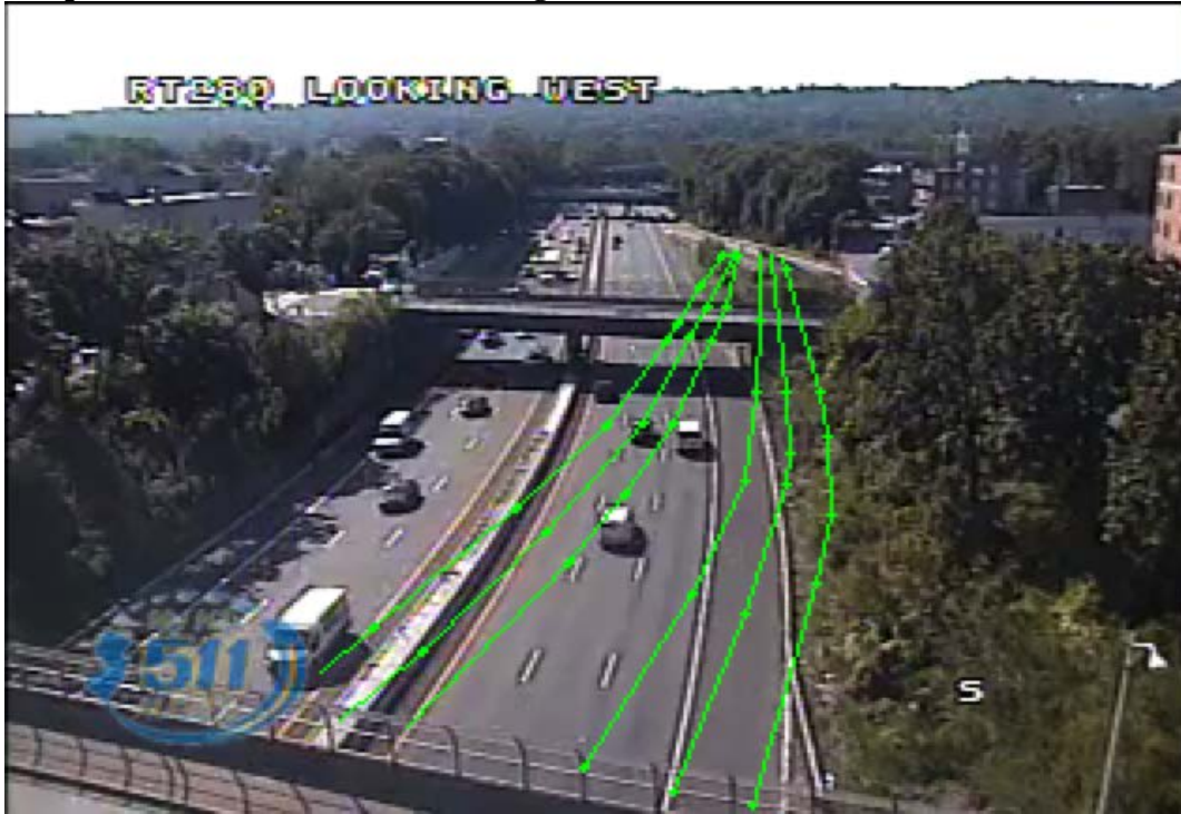
Figure 38 Sample of STLine Shifting Caused by PTZ Operations
