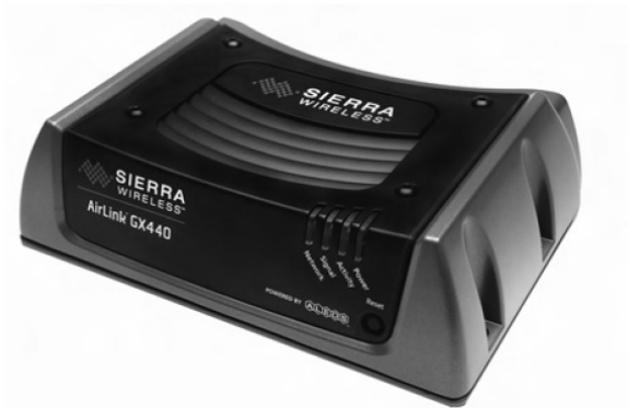
Figure 19 Cellular modem and PC remote control interface
