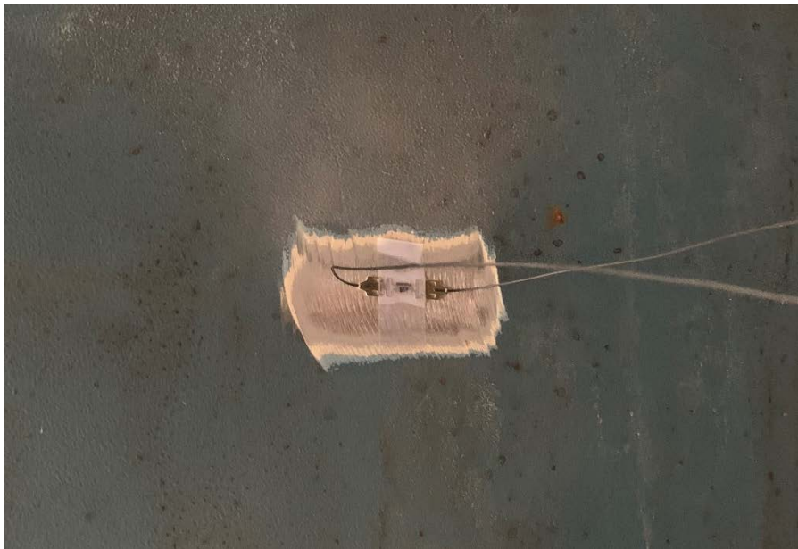
Figure 23 Paint removal to install FBG strain gage
