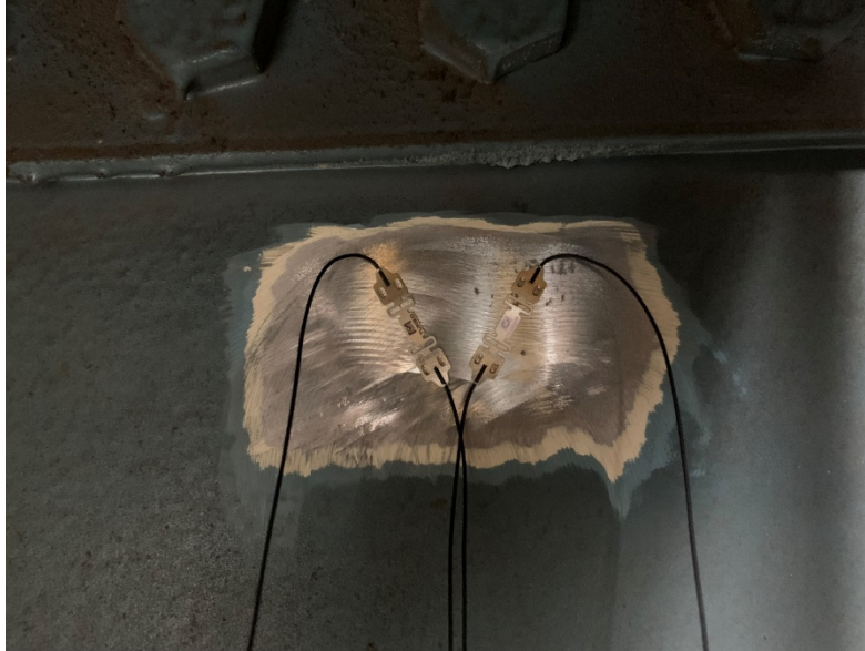
Figure 24 Typical rosette gage installation
