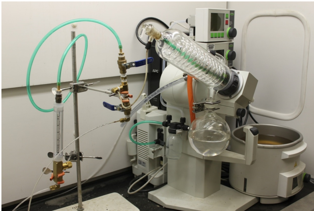
Figure 5 – Asphalt Binder Recovery Equipment at Rutgers University
