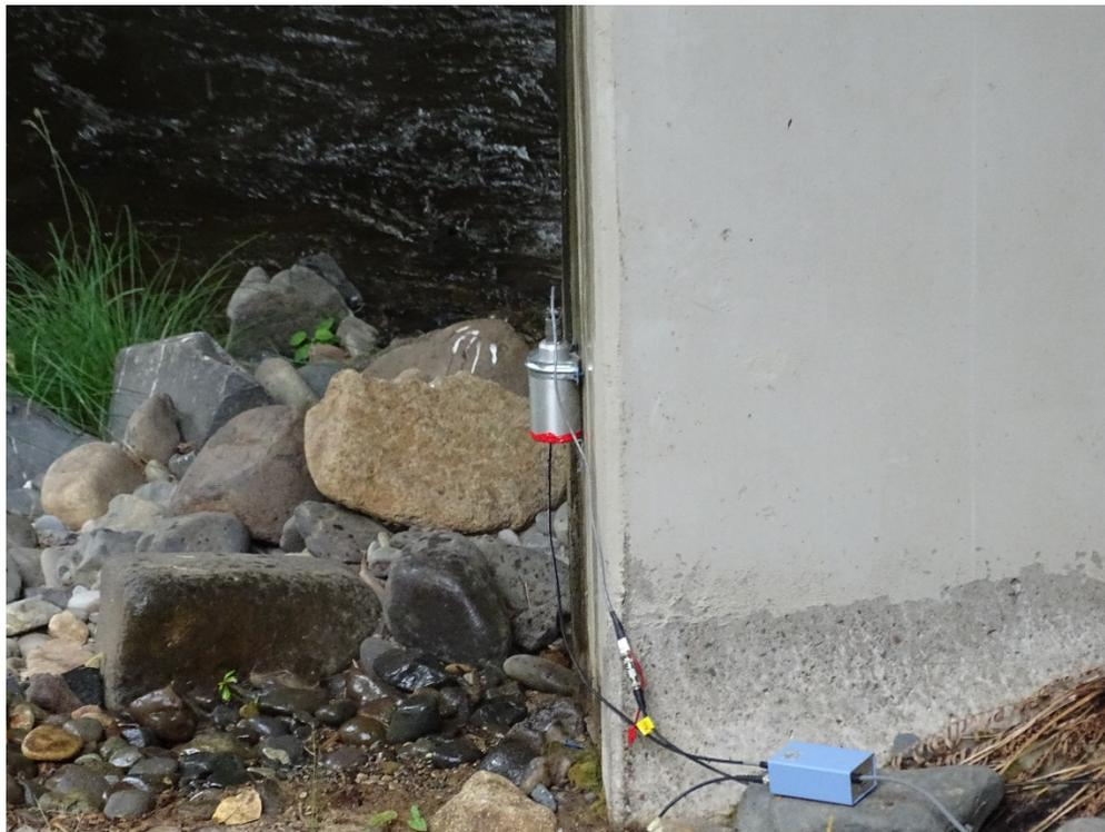
**Fig. 6. Geophone attached to the pier to measure response.**
