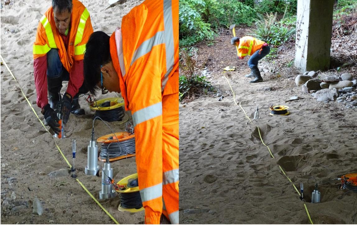
**Fig. 10. Left: setting up geophones and adjusting spacing, right: generating acoustic surface wave.**
