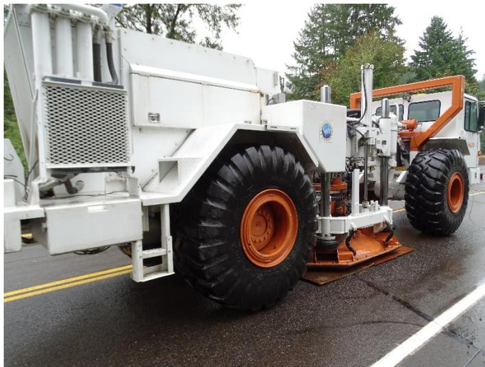
Fig. 16. T-rex loading one of the tested piers of the bridge.
