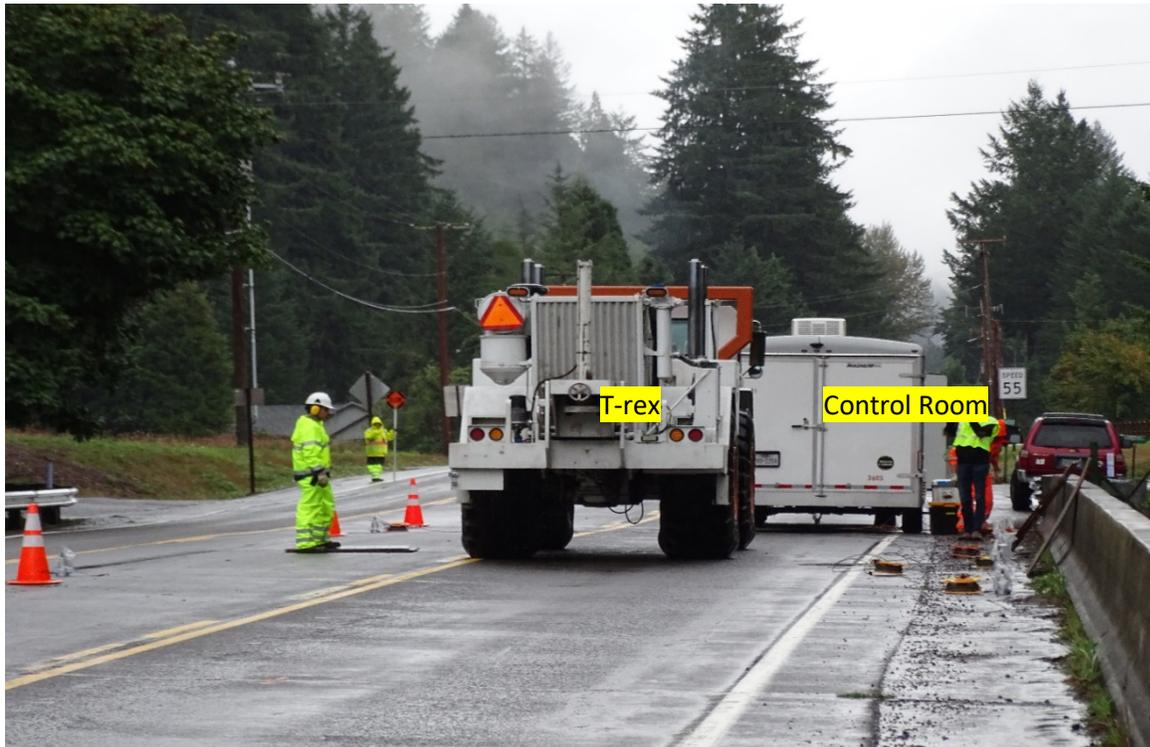
Fig. 8. T-rax and control room on the bridge ready for shaking.
