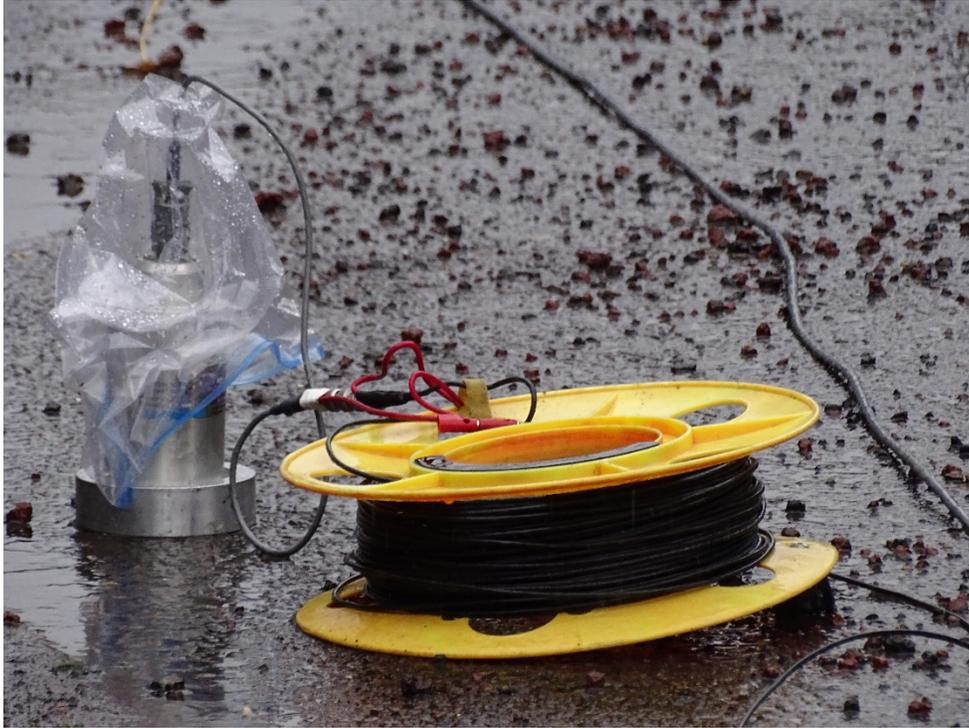
**Fig. 5. Typical geophone used for measuring response.**
