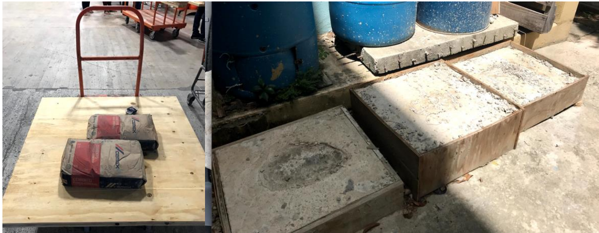
Figure 8-9 Pedestal Concrete Samples Confined with Fresh Concrete in a Wooden Formwork.
