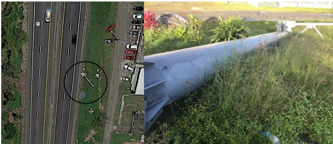
Figure 5-53: Photo of Cantilever Sign Structural Failures on The Pedestal at P-53 Location: 18°11'31.15"N; 65°53'46.75"W
