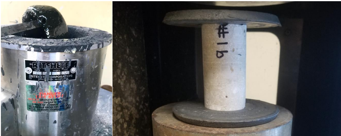
Figure 8-12 Recapping and Leveling of Cores Prior to Testing
