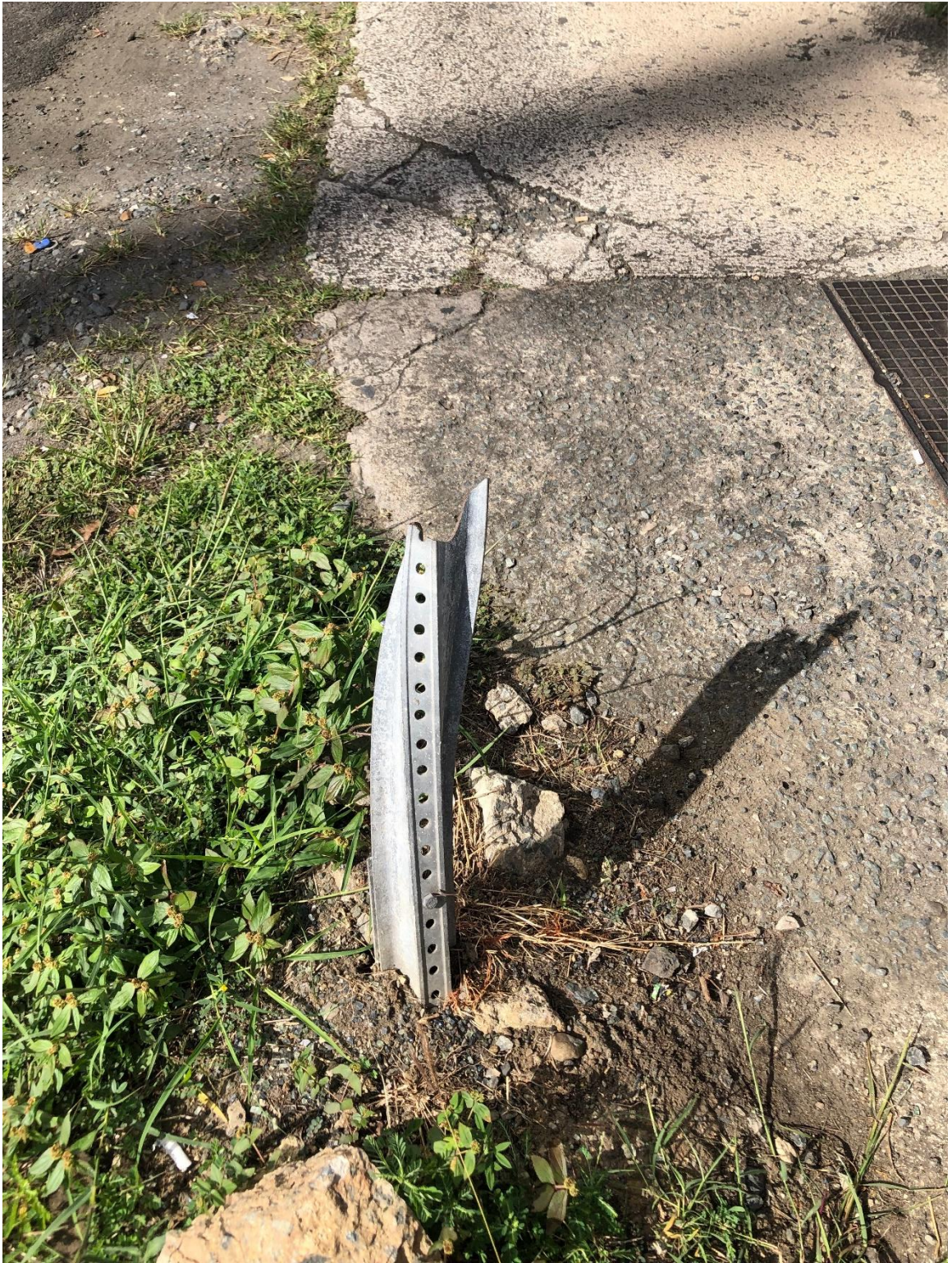
Figure 4.13: Permanent twisting deformation that led to collapse by post fracture
