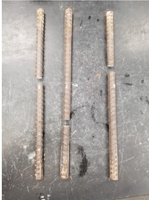
Figure 8-3: Reinforcing steel specimen after test was conducted
