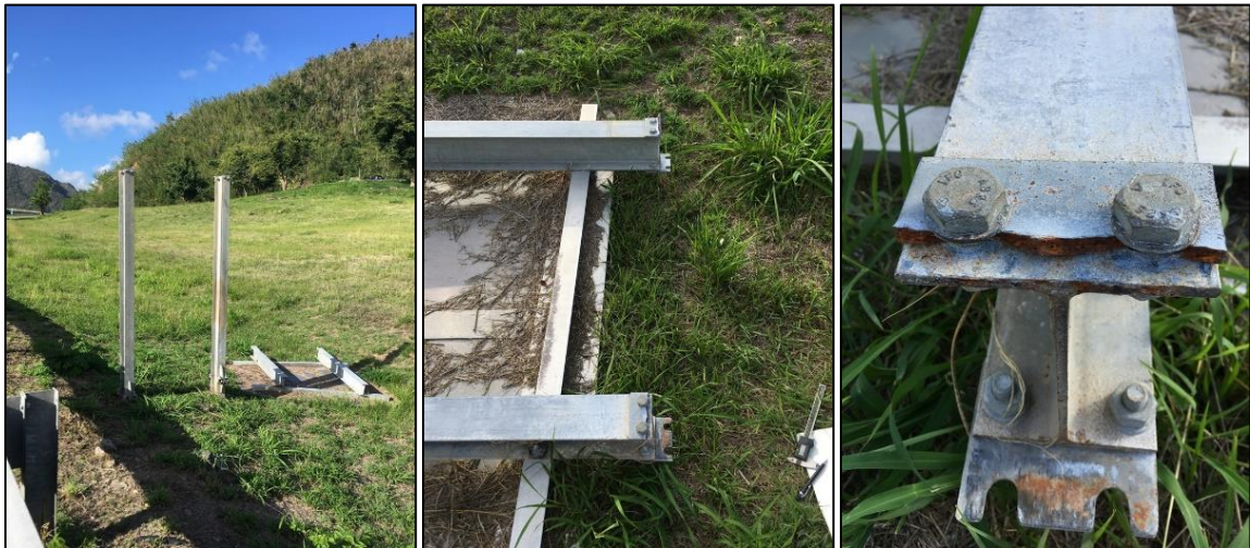
Figure 4.5: Slotted fuse plate slippage failure of Sign 7
