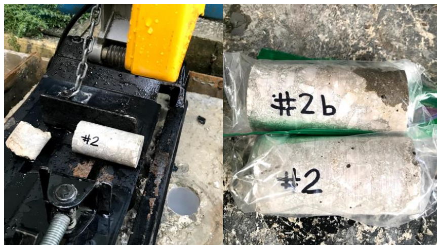
Figure 8-11 Extracted Cores, Cut and Placed Inside Plastic Bags
