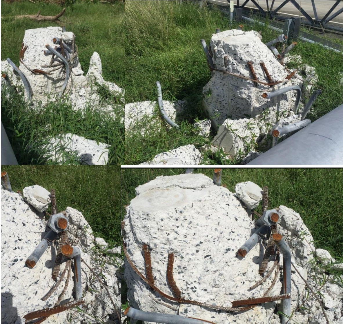
Figure 5-45: Photo of Cantilever Sign Foundation Structural Failure at P-100; with Large Deflections and Bending on the Plastic Range and Shear Fracture of the Anchor Elements, and Fractures, Detachments and Crushing of the Concrete. Anchor elements outside the confinement provided by Stirrups
