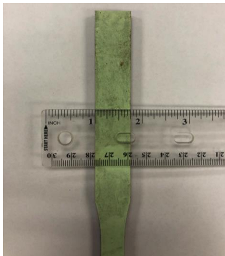
Figure 7.10: Specimen Cut Verification (2 of 2)
