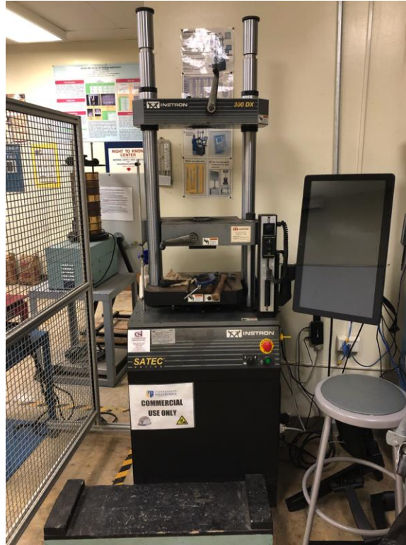
Figure 7.13: Tensile Testing Apparatus
