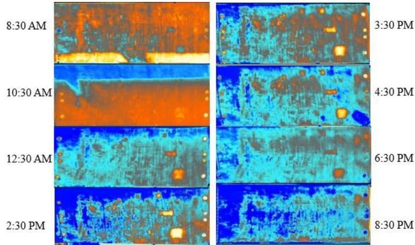
Figure 3 Concrete deck surface temperature changes during a day
