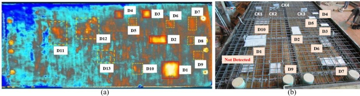
Figure 4 (a) Location of the potential delamination (D1-D13) and (b) location of the designed delamination (D1-D10; D: Delamination; CK:vertical crack)
