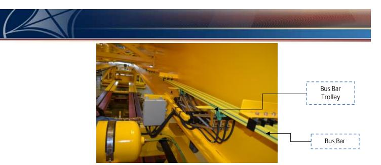
Figure 17: Top View of the Upper Carriage Assembly Highlighting the Bus Bar and Bus Bar Trolley.
