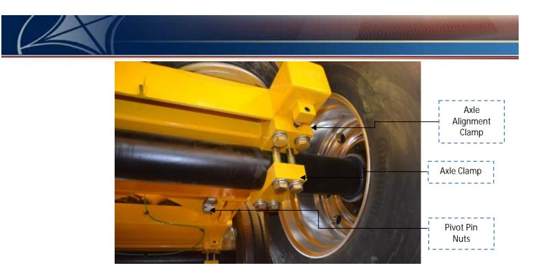
*Figure 21: Bottom View of the Lower Carriage Assembly Highlighting the Axle Clamp and Alignment System.*
