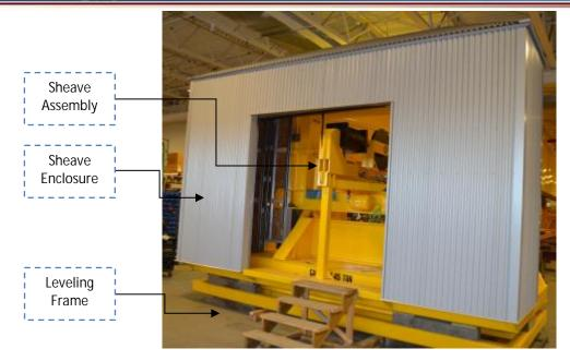
Figure 2. Sheave End Frame Assembly
