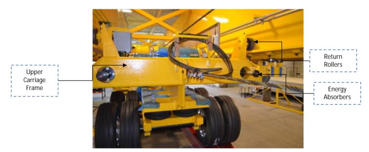
Figure 12: End View of the Carriage Assembly
