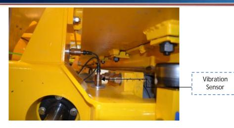
Figure 15: Vibration Sensors located on the Upper Carriage Assembly.
