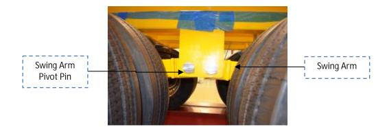
Figure 20: Side View of the Lower Carriage Assembly Showing the Swing Arms and Pivot Pins.
