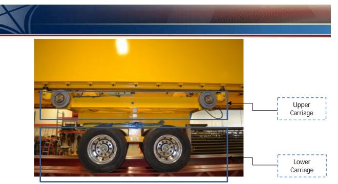
Figure 11: Side View of the Carriage Assembly
