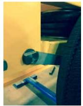
Figure 46. Axle Alignment Fixture in Place on One Side of Carriage.
