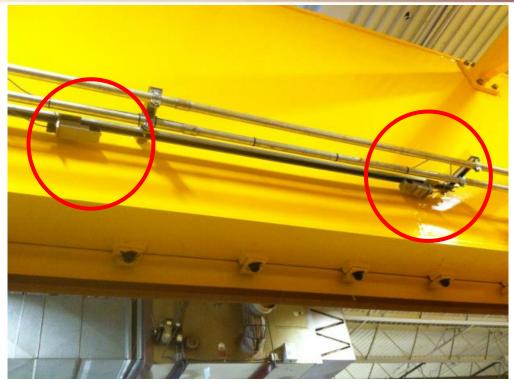
Figure 24: Optical limit switches (circled).
