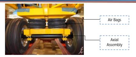
Figure 19: End View of the Lower Carriage Assembly Showing the Axle and Air Bags.
