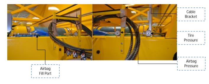
Figure 14: End View of the Upper Carriage Assembly Highlighting Pneumatic items.
