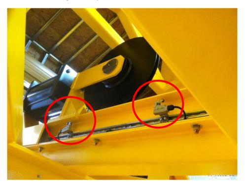
Figure 25: Tension cylinder with cylinder extend and retract switches (circled)
