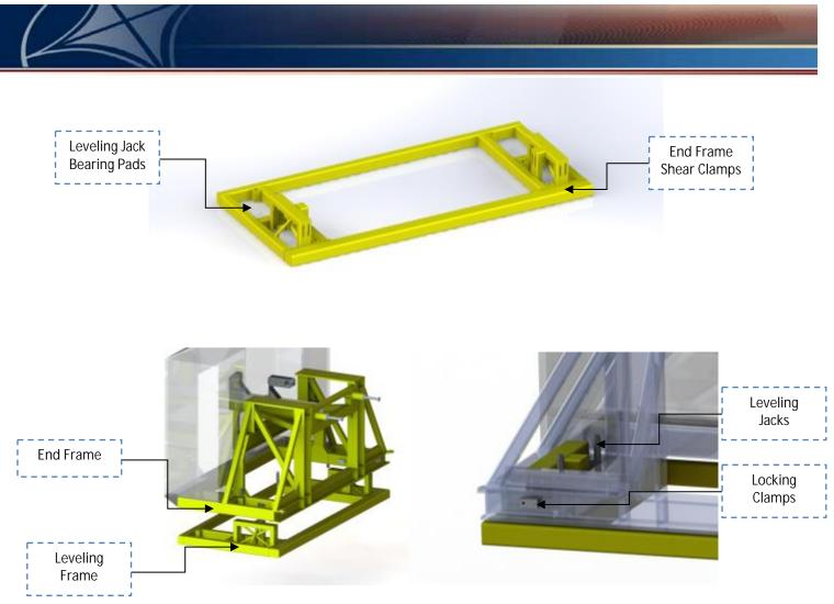
Figure 5. Leveling Frame Assembly
