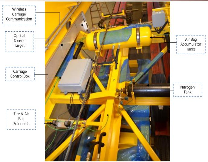
Figure 16: Top View of the Upper Carriage Assembly.
