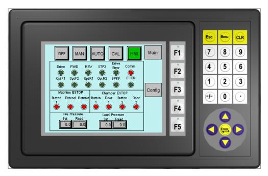
Figure 36. Main Human Machine Interface (HMI) Screen.
