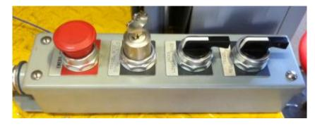
Figure 8. Rail Cart Handheld Pendent Control
