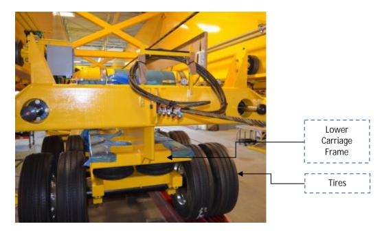
Figure 18: End View of the Lower Carriage Assembly.
