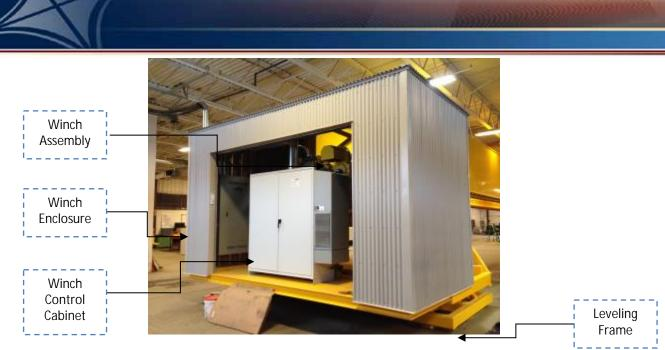
Figure 3. Winch End Frame Assembly Showing Winch, MDP, and Winch Controller
