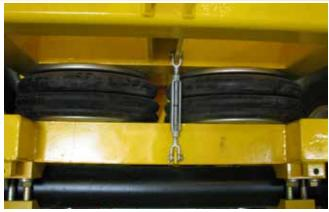
Figure 47. Turnbuckle Supporting Axle and Swingarm.
