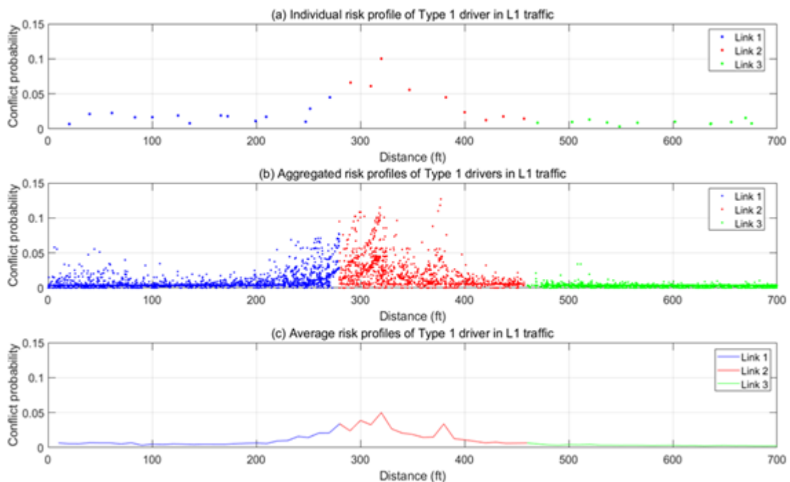
Figure 28. Risk profile of the sample roadway section.
