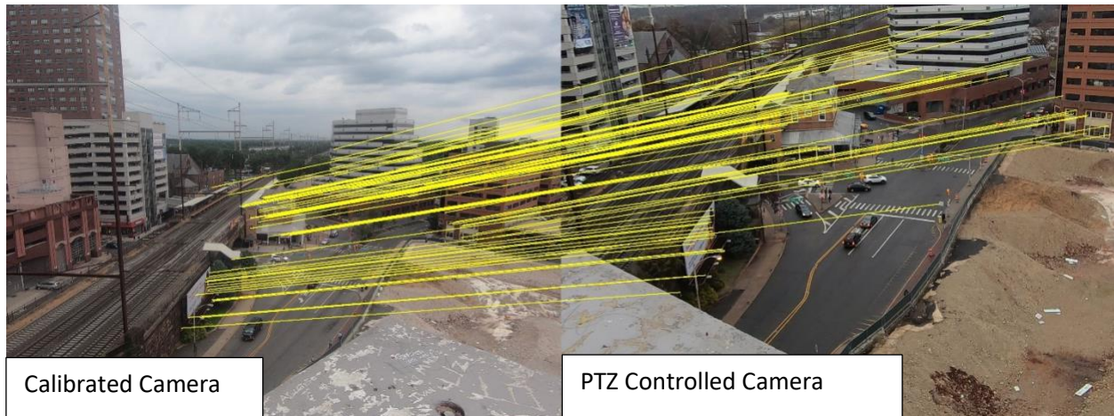
Figure 13. Feature matching between the original image and Rotated-Zoomed image
