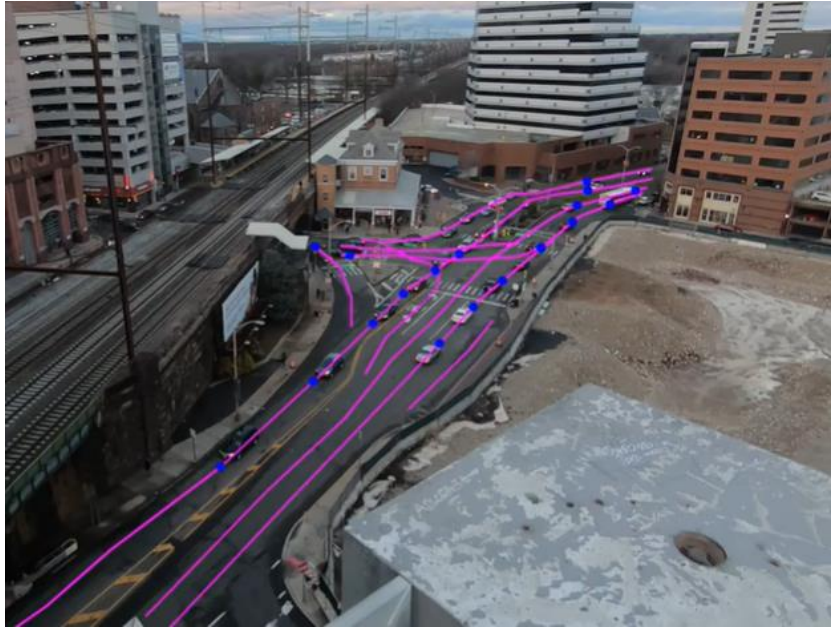
Figure 3. Scanline-Based Vehicle Trajectory Detection
