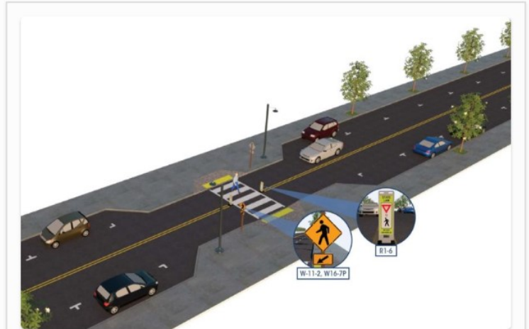
Crosswalk Visibility Enhancements
