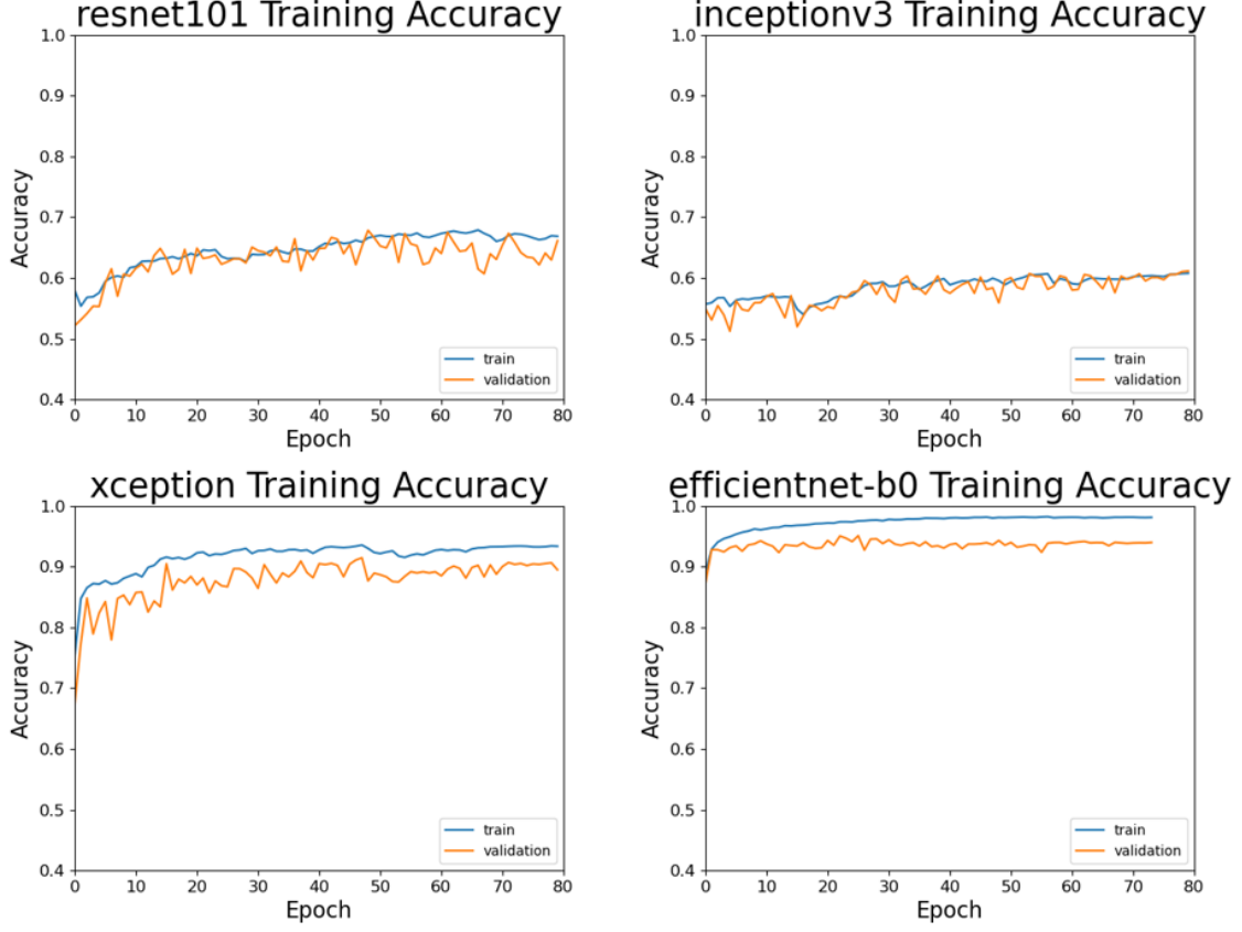
Figure 5: Training (blue) and validation (orange) accuracy curves for ResNet101 (top left), Inception-V3 (top right), Xception (bottom left), and EfficientNet-b0 (bottom right).
