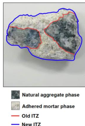
Figure 1: Meso-structure of material phases in an RCA particle
