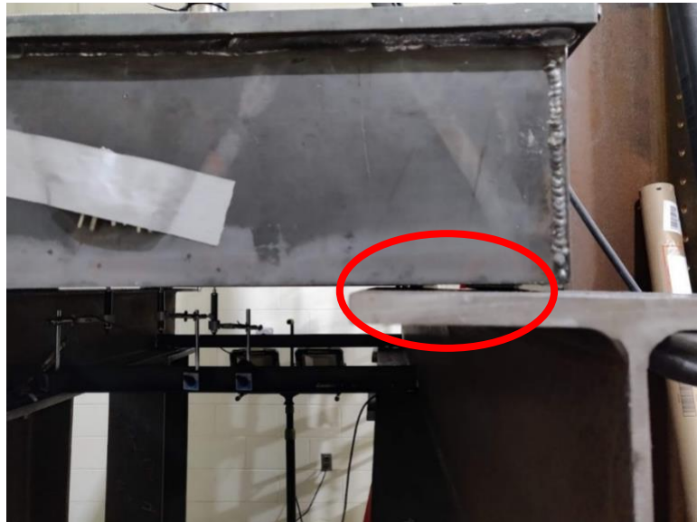
Figure 5 Straight-on view of shims
