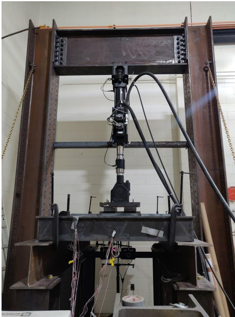
Figure 7 Overall test setup – end view
