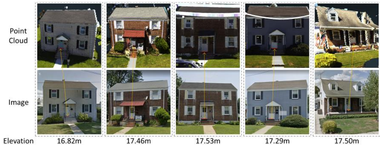
Figure 6 Examples of extraction of lowest floor elevation
