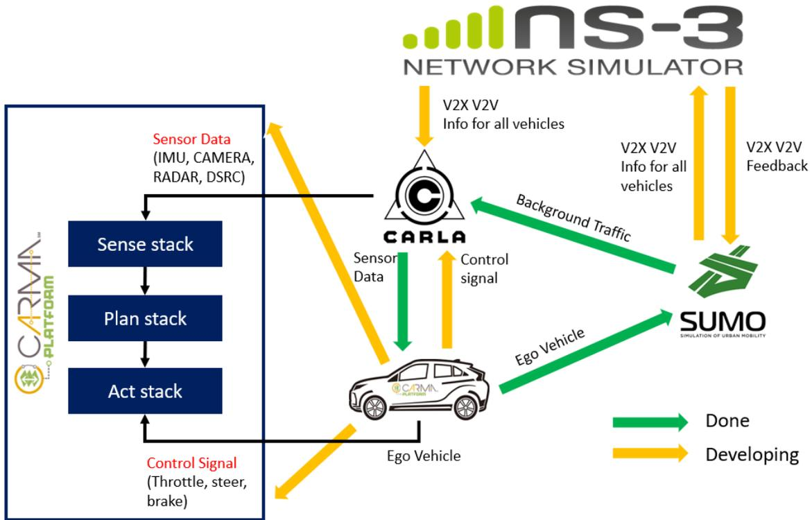
Figure 4.2: Structure of the digital twin.
