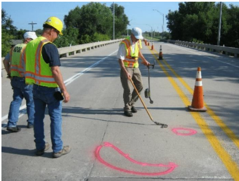
Figure 2. Chain Dragging Test (Source: www.researchgate.net ).
