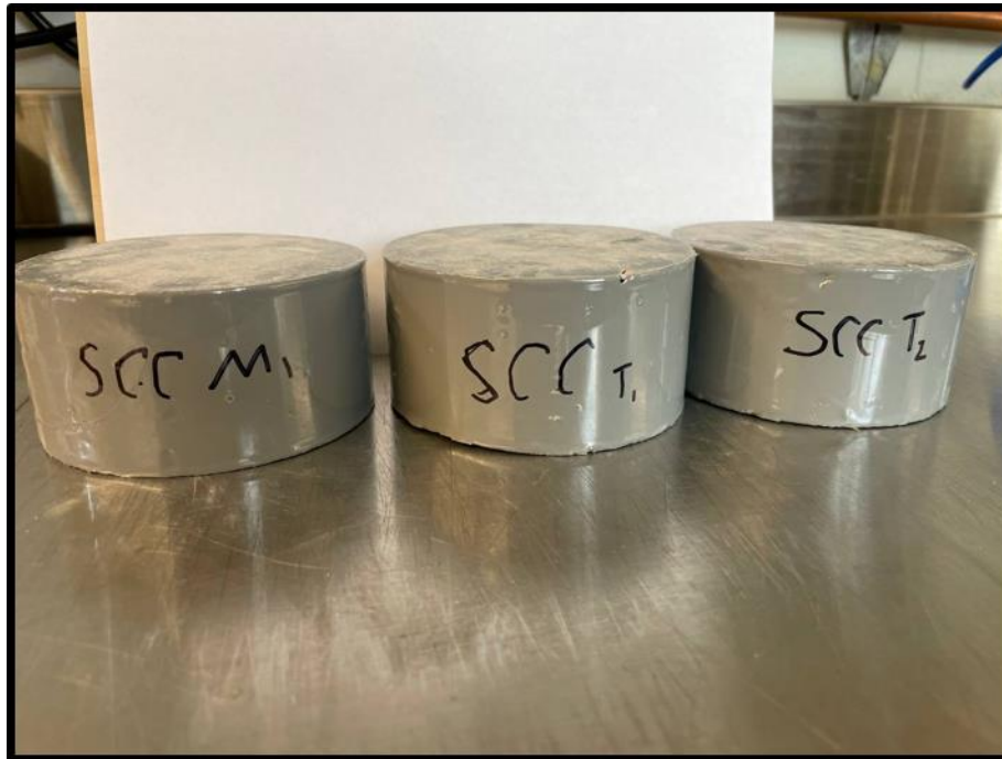
Figure 4: Cut and epoxy coated specimens before testing
