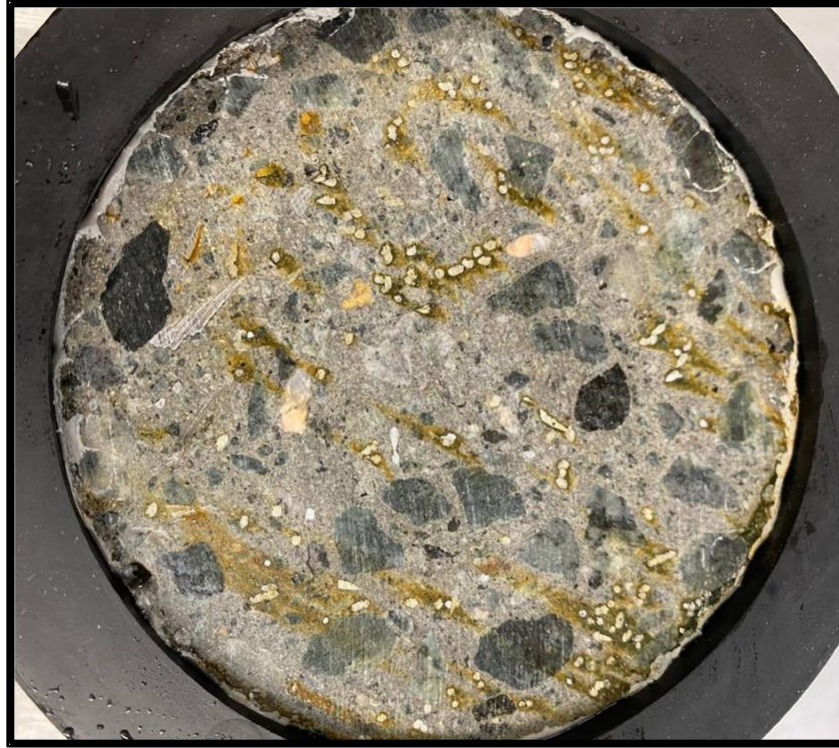
Figure 7: SC-HyFRC specimens after removing from the cell
